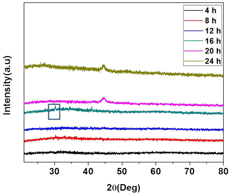
Figure SI 6. XRD ptteren of NiCoFe alloy mutishell hollow spheres at diffrent reaction time.
