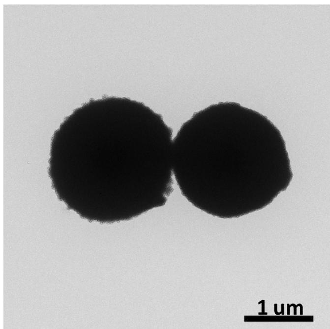
**Figure SI 1.** TEM image of NiCoFe alloy spheres without using urea.
