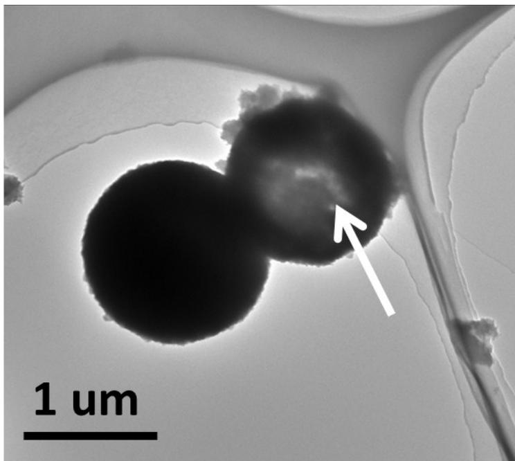
**Figure SI 3.** TEM image of NiCoFe alloy spheres without using citric acid.
