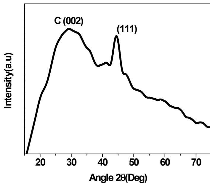
Figure SI 7. XRD ptteren of NiCoFe alloy mutishell hollow spheres after 24 hours reaction time.
