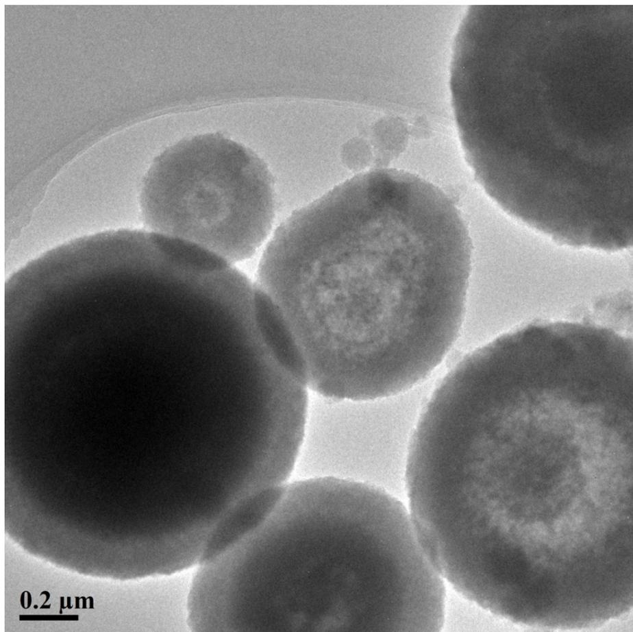
**Figure SI 5.** TEM image of NiCoFe alloy spheres at the reaction time of 24 hours.
