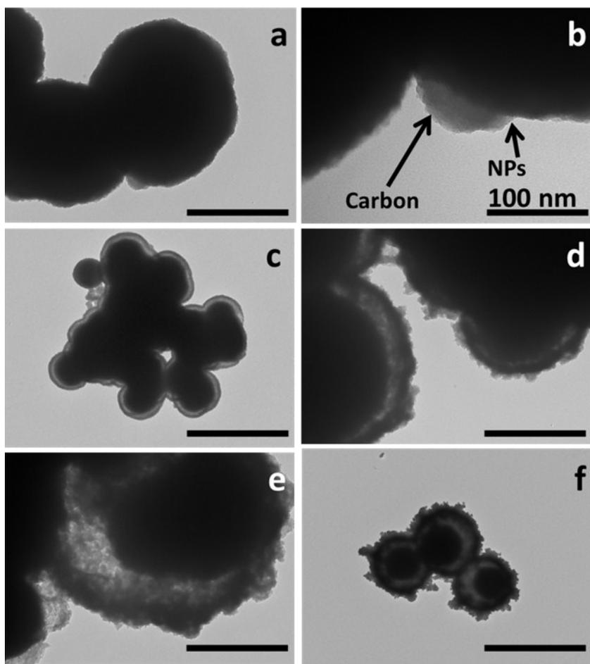
**Figure SI 4.** TEM image of NiCoFe alloy spheres at different time of reaction (scale bar is 500 nm).
