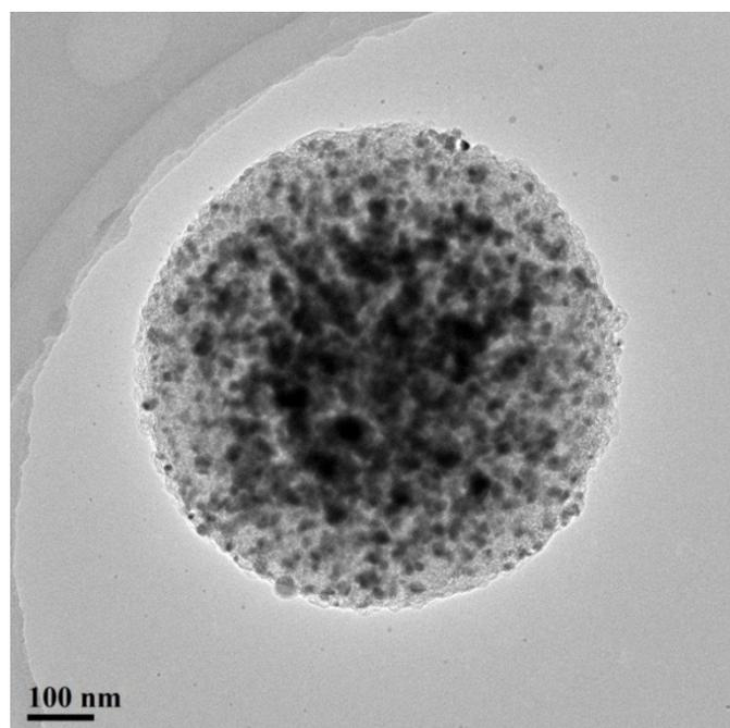
**Figure SI 2.** Enlarged TEM image of NiCoFe alloy spheres without using urea.
