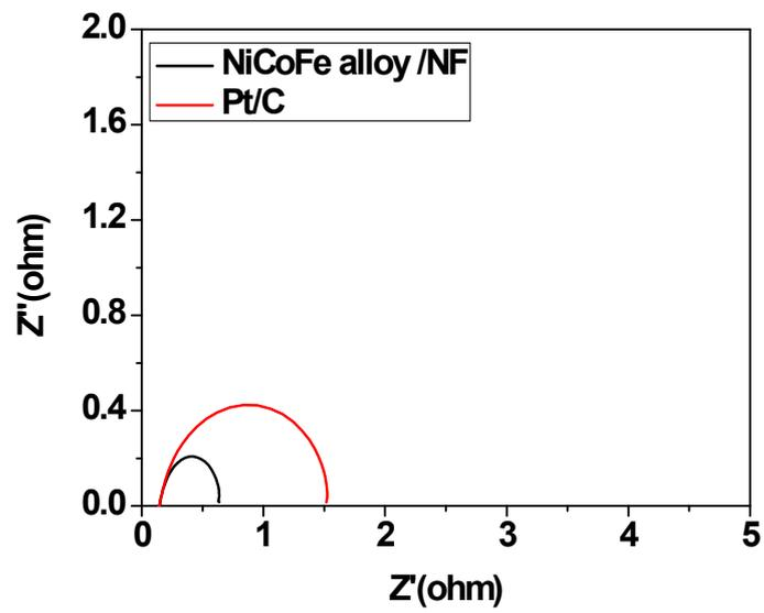
**Figure SI 10.** Electrochemical impedance spectra of NiCoFe alloy and Pt/C.
