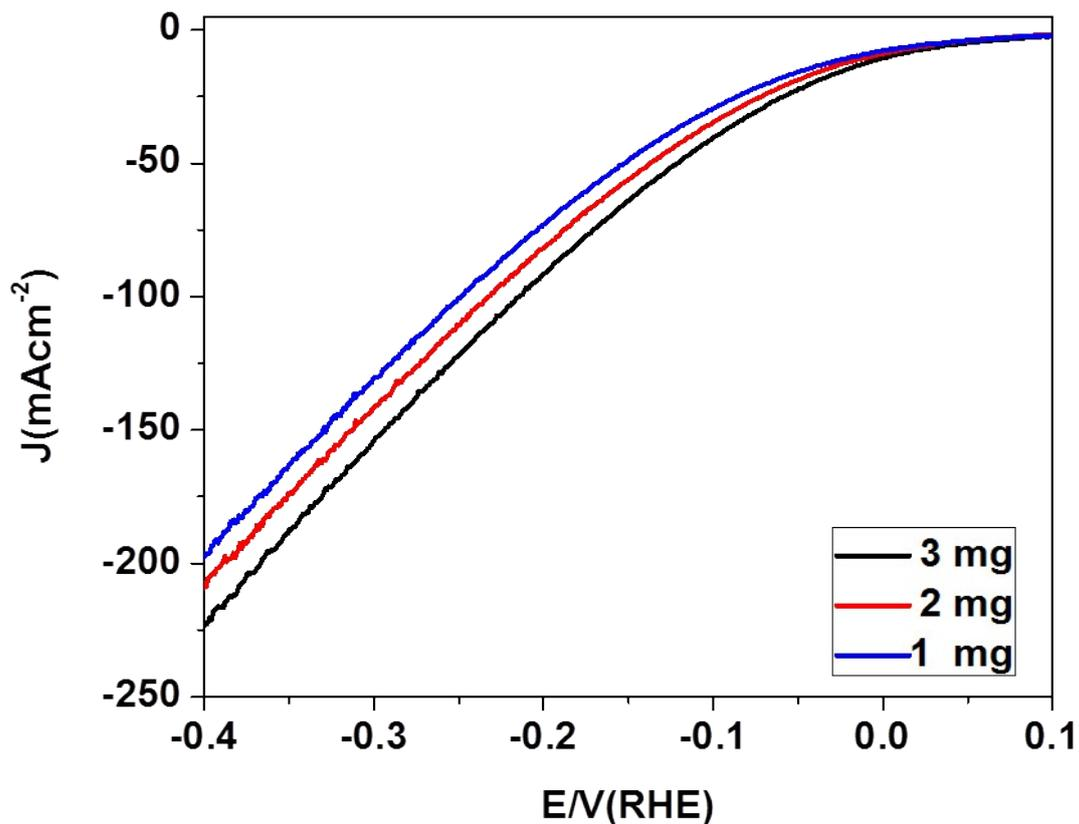
**Figure SI 8.** Polarization curve of NiCoFe alloy hollow spheres at the different loading of catalyst.
