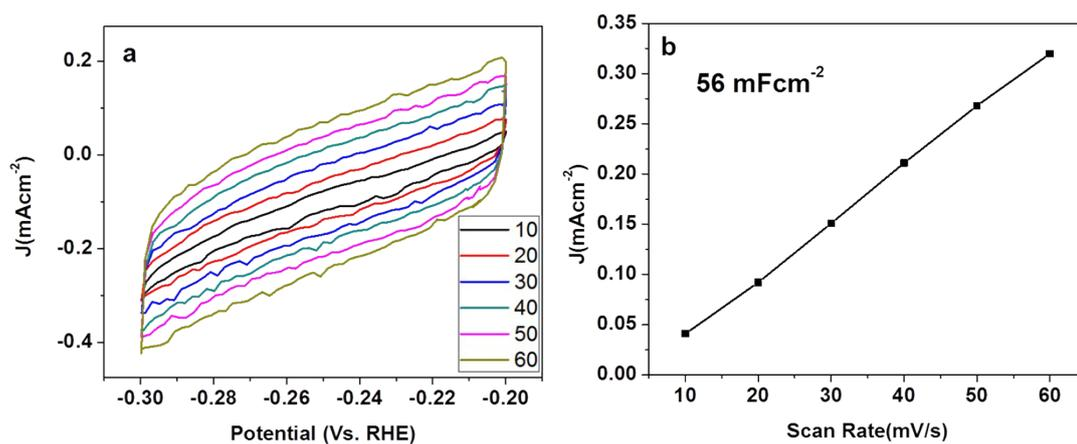
**Figure SI 9.** Cyclic voltammograms (CV) curves NiCoFe alloy multishell hollow spheres (a), and current density as a function of scan rate (mV/s) derived from (a) of NiCoFe alloy multishell hollow spheres (b).
