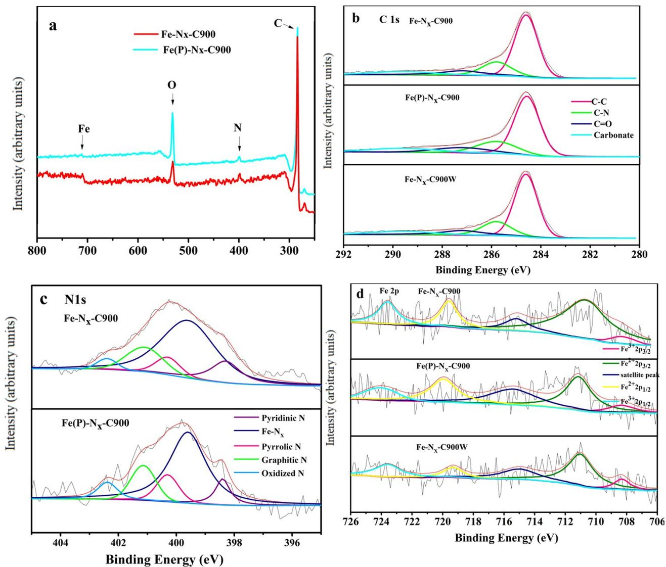
Fig. S3 (a) XPS survey spectra of Fe-N<sub>x</sub>-C900 and Fe(P)-N<sub>x</sub>-C900 (Pour Fe loading caused by multi-time washing after acid treatment), (b) N 1s and (c) C 1s spectra of Fe-N<sub>x</sub>-C900 and Fe(P)-N<sub>x</sub>-C900, and (d) Fe 2p spectra of Fe-N<sub>x</sub>-C900AH, Fe(P)-N<sub>x</sub>-C900 and Fe-N<sub>x</sub>-C900W (Fe-N<sub>x</sub>-C900W: acid-treated catalyst without 300 °C annealing in vacuum).
