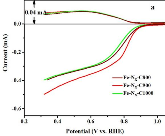
Fig. S5. (a) RRDE of catalysts at a sweep rate of  $10 \text{ mVs}^{-1}$  under rotating speeds of  $1600 \text{ rpm}$  in  $\text{O}_2$  saturated  $0.1\text{M KOH}$
