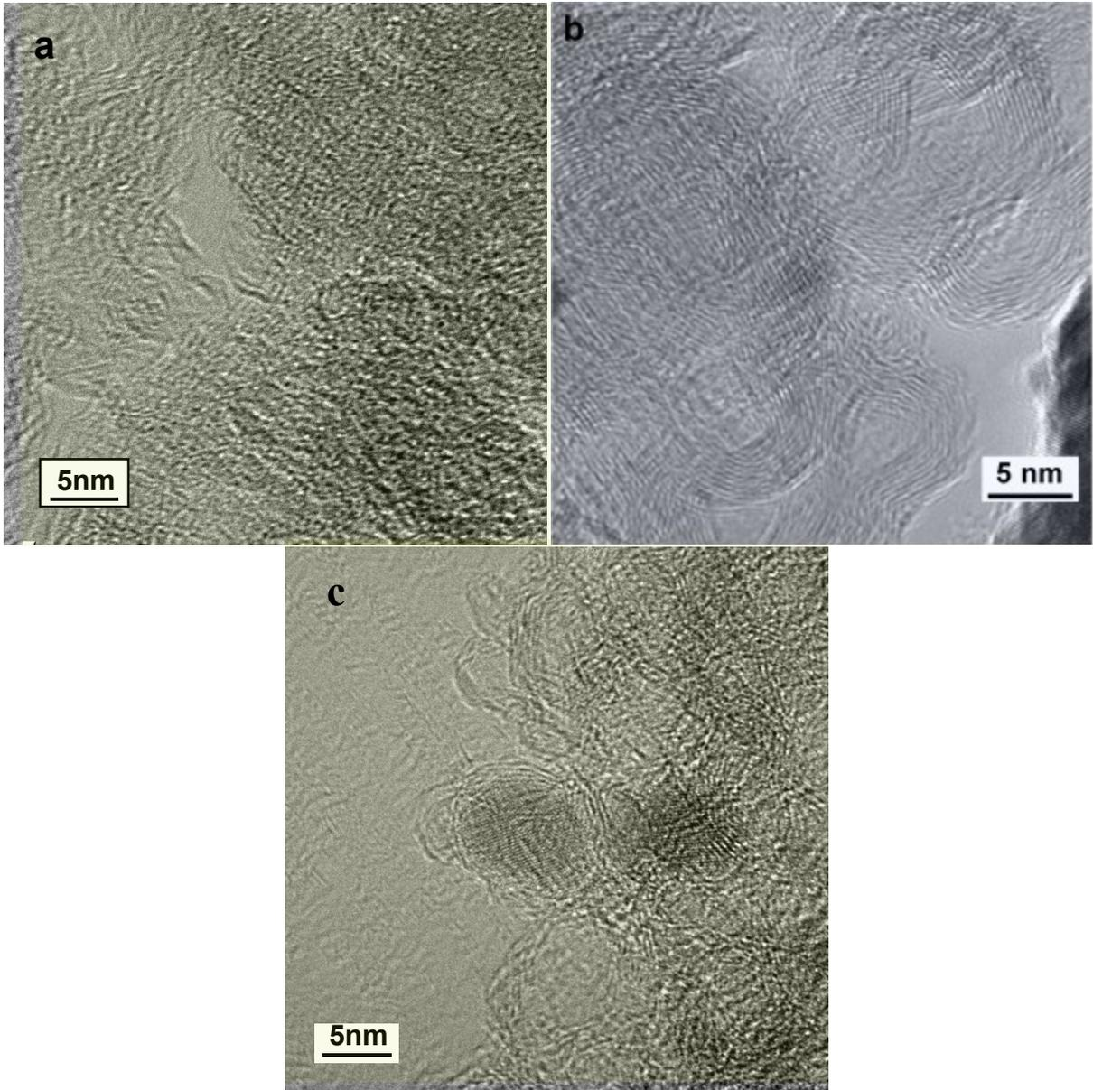
Fig. S2 HRTEM images of (a) Fe-N<sub>x</sub>-C700, (b) Fe-N<sub>x</sub>-C1100, (c) Fe-N<sub>x</sub>-C900HCl.
