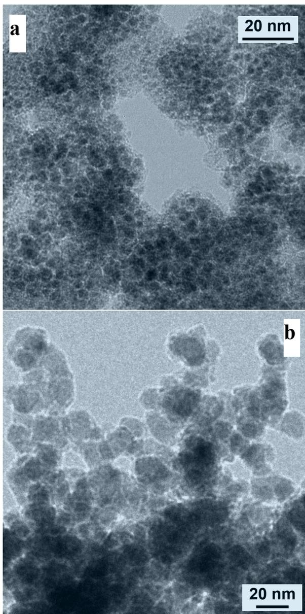
Fig. S1 TEM images of core-shell precursors: (a)  $\text{Fe}_3\text{C}@$ NDC700 and (b)  $\text{Fe}_3\text{C}@$ NDC1100.
