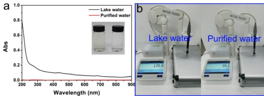
**Fig. S10** (a) The absorption spectra of lake water and purified water (Insert: photo of lake water (left) and purified water (right)). (b) Conductivity photograph of lake water and purified water.
