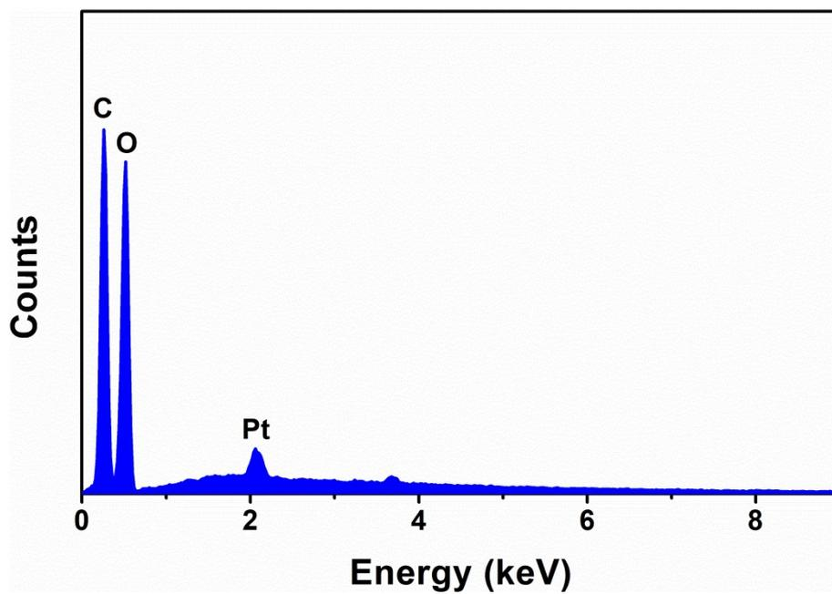
**Fig. S3** Cross-section EDS of the pristine wood.
