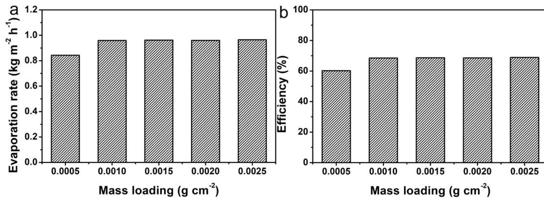
**Fig. S7** Evaporation rate and efficiency of CS-wood device with different mass loadings of candle soot nanoparticles.
