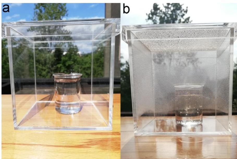
**Fig. S8** Outdoor solar seawater desalination by CS-wood device under natural sunlight.
