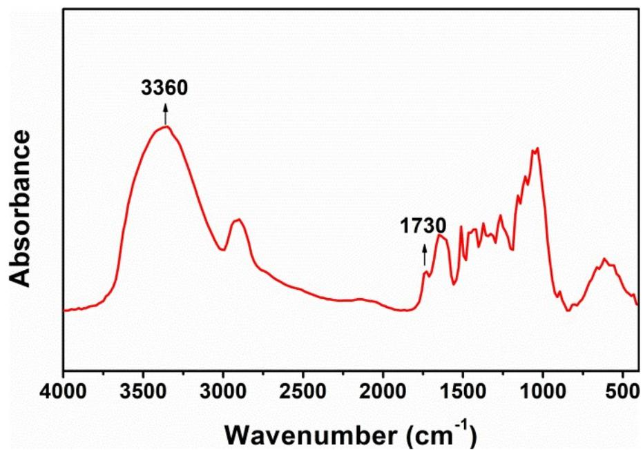
Fig. S4 FTIR of the wood substrate.
