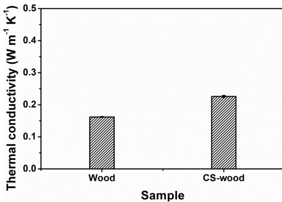
Fig. S6 Thermal conductivities of the pristine wood and CS-wood.
