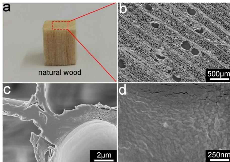
**Fig. S1** (a) Photo image of natural wood. (b-d) Cross section SEM images of natural wood under different amplification.
