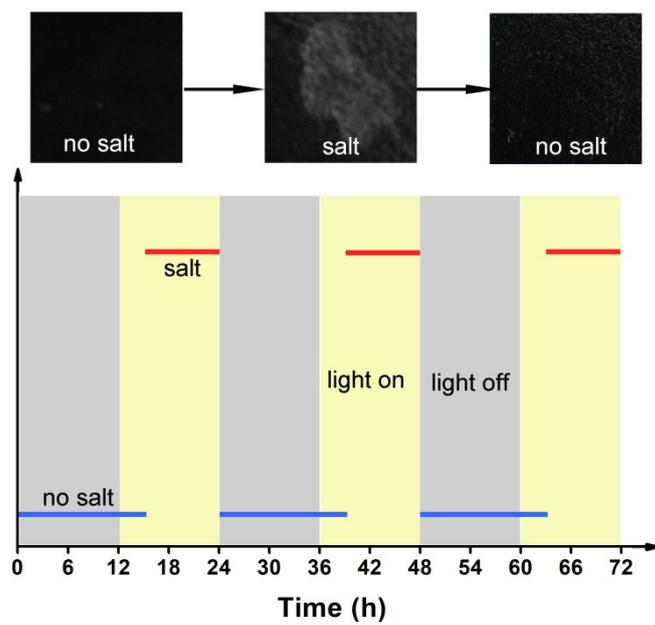
**Fig. S9** The salt generates under illumination and dissolves automatically under dark conditions.
