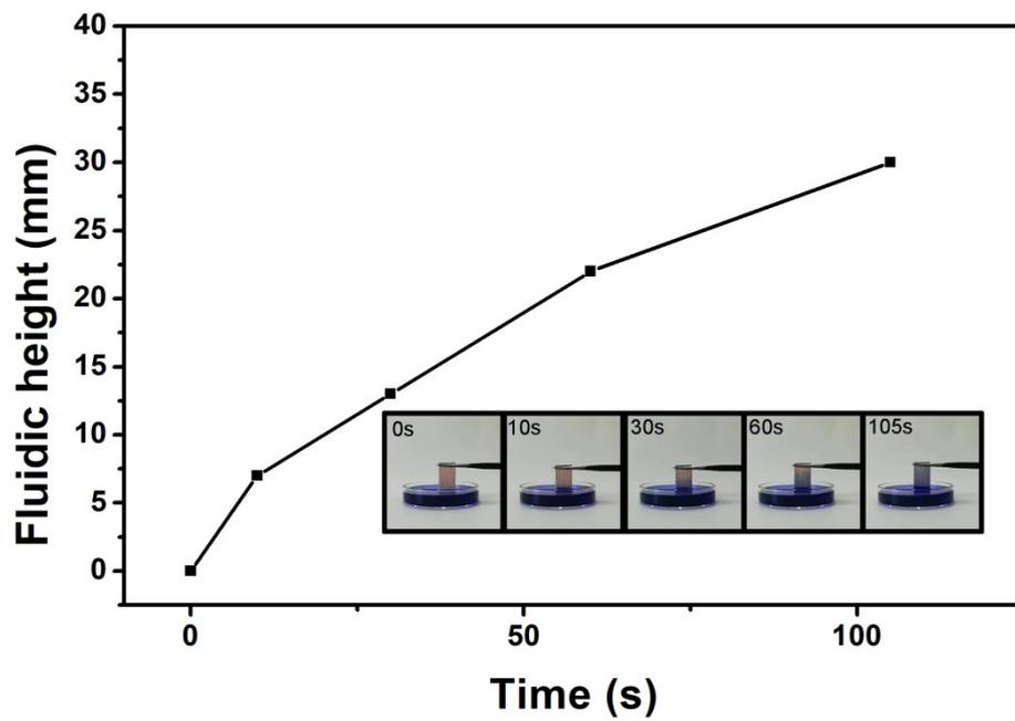
**Fig. S5** The transportation of the methyl-blue aqueous solution along wood.
