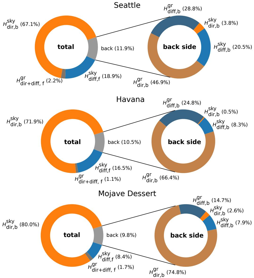
Figure S.4: (left) Different annual radiant exposure components for a bifacial solar cell in Seattle, Havana and Mojave Dessert. (right) Detailed picture for the back side. Simulated with module spacing  $d = 10$  m, module tilt  $\theta_m = 42^\circ$ , module height  $h = 0.5$  m and albedo  $A = 30\%$ .
