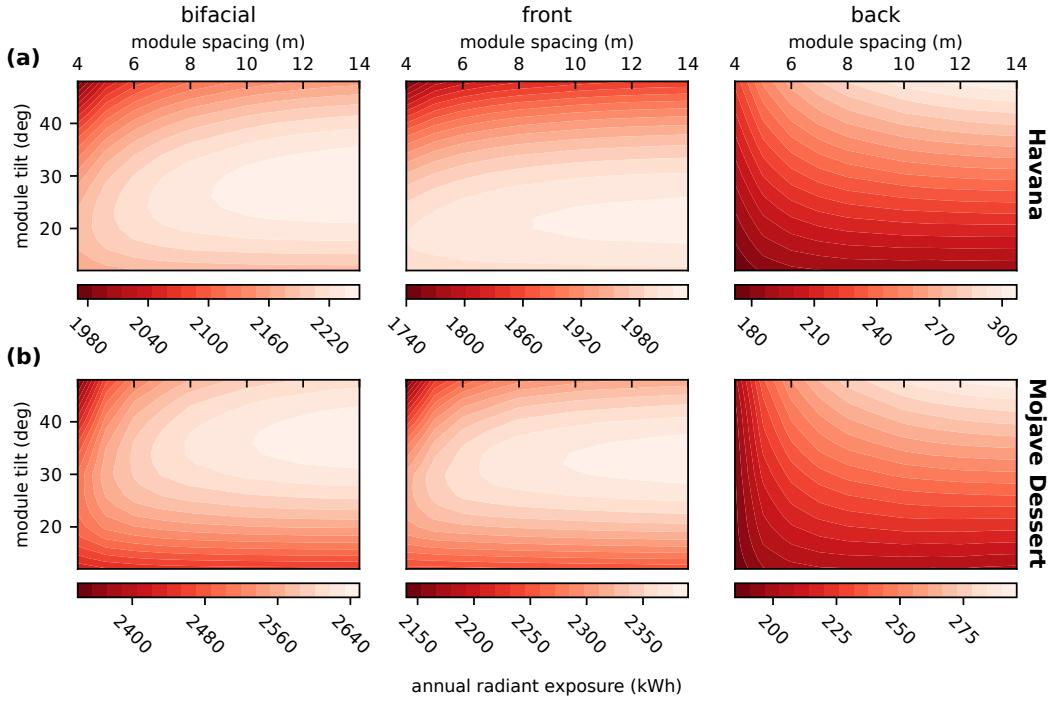
Figure S.5: Annual radiant exposure for bifacial modules and the contributions from front and back sides in a large PV field as a function of module spacing  $d$  and module tilt  $\theta_m$ . Results are shown for Havana (top row) and Mojave Dessert (bottom row). The annual radiation yield is calculated using eq. (4) with  $\eta_f = \eta_b = 1$ . Simulated with m module height  $h = 0.5$  m and albedo  $A = 30\%$ .
