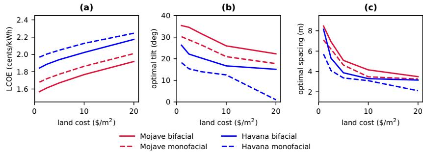
Figure S.6: Results of the optimisation for different land cost scenarios in Mojave Dessert (red lines) and Havana (blue lines): (a) lowest LCOE and (b) optimal module tilt and (c) optimal spacing. Simulations with albedo  $A = 30\%$ , module height  $h = 0.5$  m and peak power costs  $c_p$  1000 \$/kWh.
