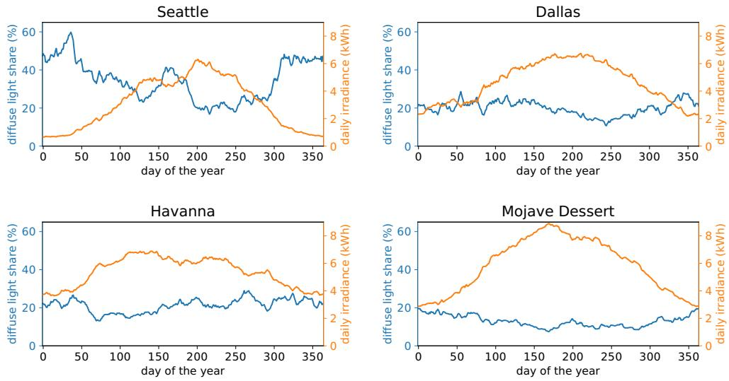
Figure S.3: 30 days moving average of isotropic diffuse light share (blue curve) and daily global horizontal irradiance (orange curve) for the typical meteorological year.
