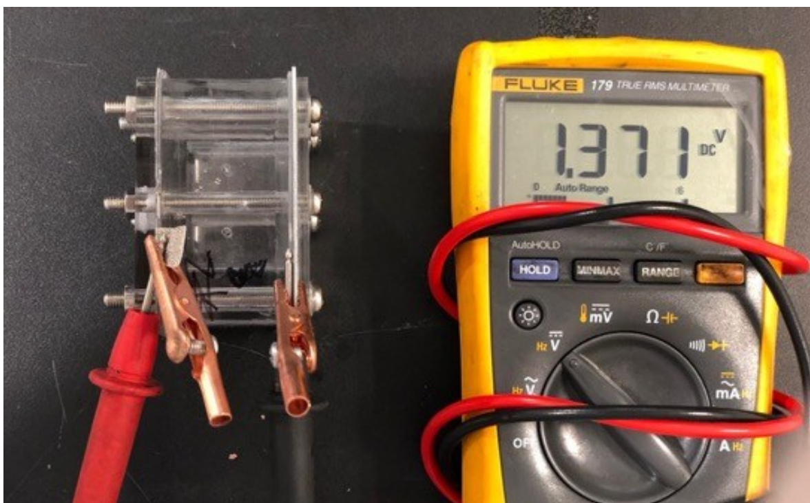
Fig. S9. Digital image of the aqueous Zn-air battery using h -FeCo alloy/ N -CNFs air cathode.
