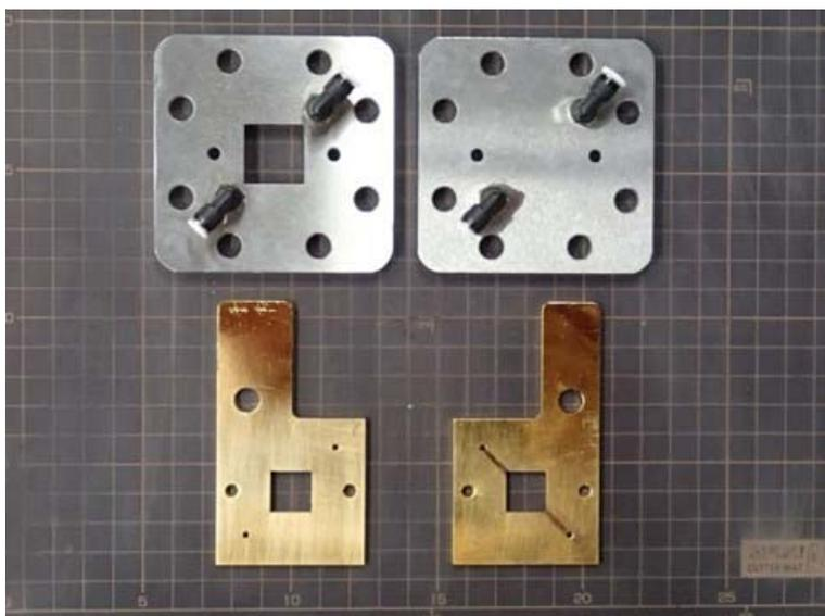
**Figure S15.** A photo of a planar-type dual-compartment stainless-steel reactor with irradiation area of  $2.0 \text{ cm}^2$  ( $1.4 \times 1.4 \text{ cm}^2$ ).
