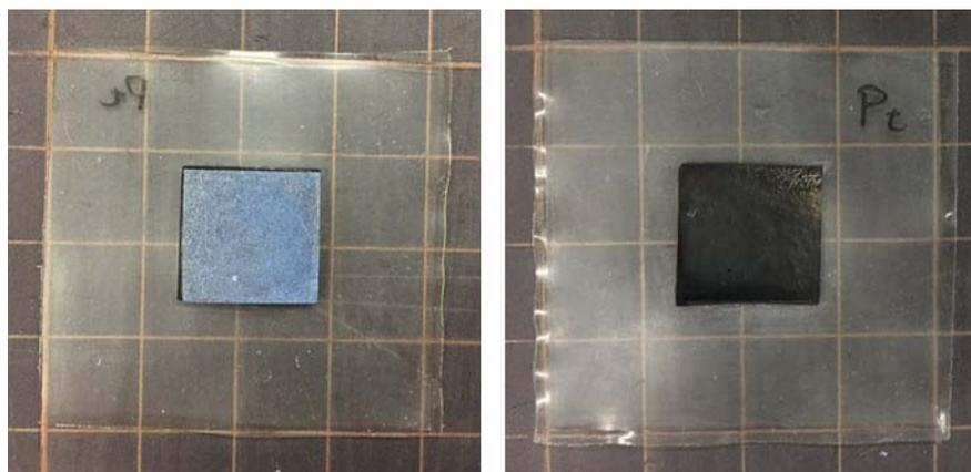
**Figure S10.** Photos of a membrane electrode assembly. The left-side photograph shows the side of the ionomer-coated oxide layers on the titanium microfiber felt. The right-side photograph shows the side of the ionomer-mixed Pt/CB film as an H<sub>2</sub>-evolving cathode.
