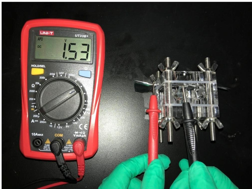
**Figure S17.** Photograph of the battery with an open-circuit voltage of  $\sim 1.53$  V.
