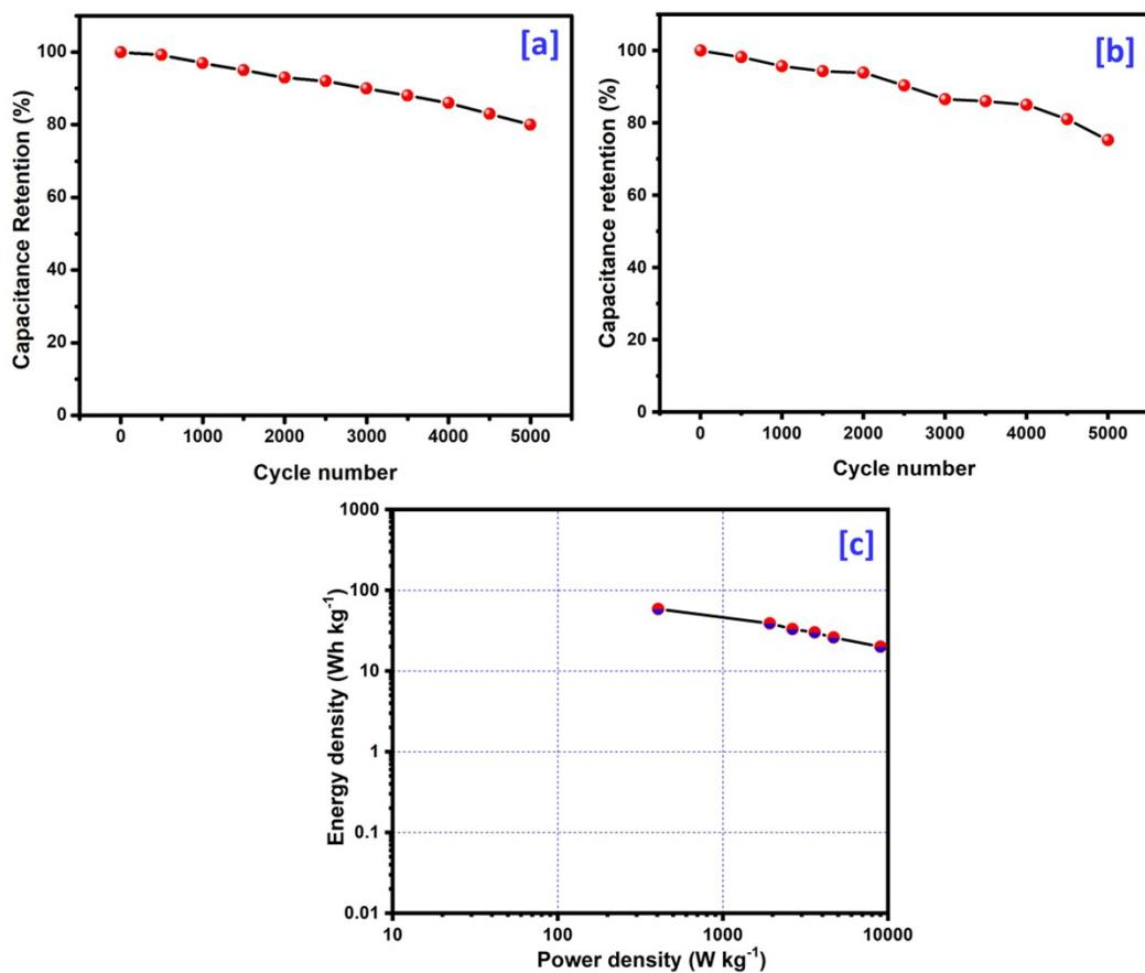
**Figure S7.** (a) Cyclability profile of CL-700 symmetric three electrode cell for 5000 cycles at 5 A/g current density of CL-700 in 1 M  $\text{Na}_2\text{SO}_4$  + KI redox additive electrolyte (b) Cyclability profile of CL-700 symmetric two electrode cell for 5000 cycles at 5 A/g current density of CL-700 in 1 M  $\text{Na}_2\text{SO}_4$  + KI redox additive electrolyte (c) Ragone plot of CL-700 symmetric cell in 1 M  $\text{Na}_2\text{SO}_4$  + KI redox additive electrolyte.
