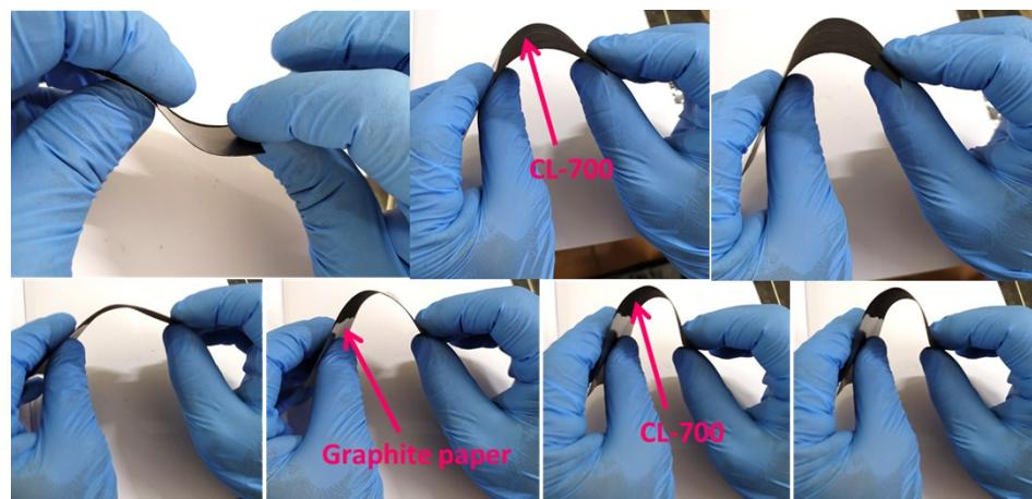
**Figure S5.** Mechanical stability testing for CL-700 electrode material with different bending angle in both directions.
