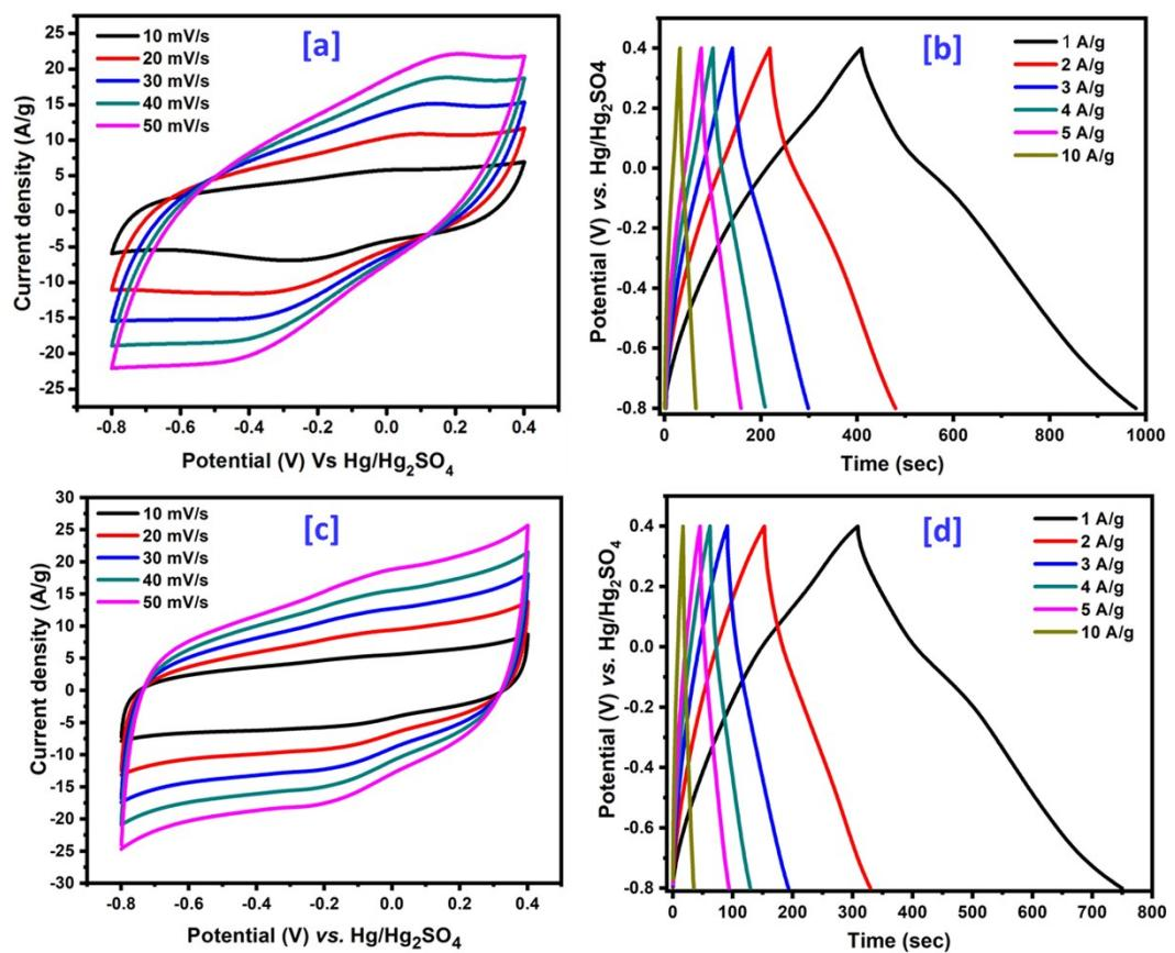
**Figure S3.** CV and CD profile of (a-b) CL-600 and (c-d) CL- 800.
