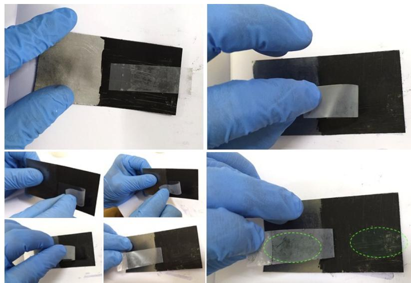
**Figure S4.** Tape testing for CL-700 electrode material.
