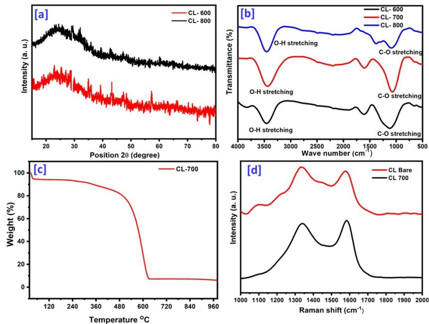
**Fig. S2** (a) XRD pattern of CL-600 and CL-800, (b) FT-IR spectrum of all the three activated carbons, (c) TGA plot for CL-700 and (d) Raman spectra for CL- bare and CL-700
