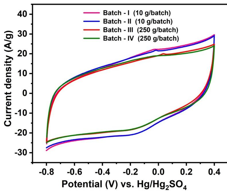
**Figure S6.** CV profile of CL-700 electrode materials prepared at different batch.
