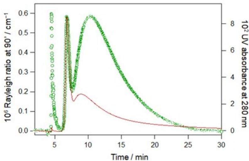
**Figure S4.** AF4-MALS fractograms of PACaL6 micelles in 50 mM NaCl aqueous solutions (pH = 3.0). The green points and red lines are the Rayleigh ratio at 90° and UV absorbance at 280 nm.
