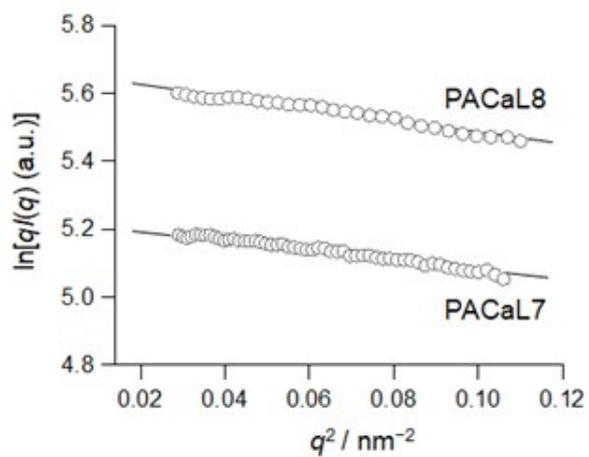
**Figure S3.** The cross-sectional Guinier plot for PACaL7 and 8 providing the cross-sectional radius.
