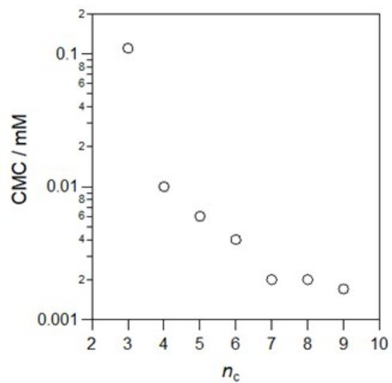
**Figure S5.** Alkyl chain dependence of critical micelle concentration (CMC) .
