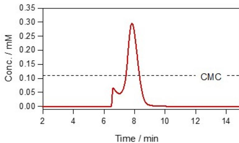
**Figure S6.** The concentration profile determined by UV absorbance in AF4-MALS fractograms of PACaL3 micelles in 50 mM NaCl aqueous solutions (pH = 3.0).
