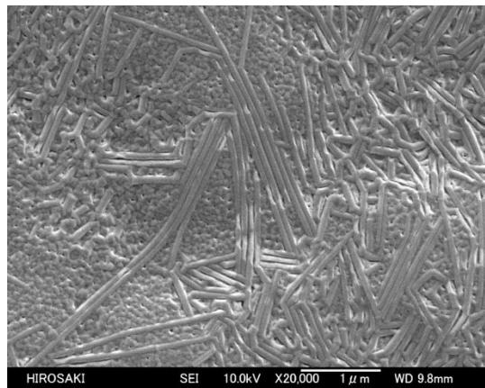
Fig. S8 SEM image of the surface structure of a mixture of **I-5** (50 mol%) and **I-7** (50 mol%).
