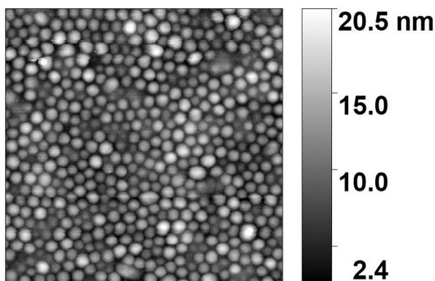
**Figure S7.** AFM height image of the 68-26k PS-P2VP film (55 nm) after thermally annealing for 3 hr at 150°C in the absence of shear forces. Image is of a 1 x 1  $\mu\text{m}$  area. The P2VP phase was Pt infiltrated to improve contrast between polymer domains.
