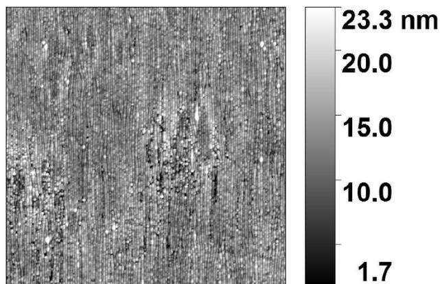
**Figure S4.** AFM height image showing the representative nanowire morphology of a shear-aligned 48-14 PS-P2VP film that is thicker than the optimum (63 nm instead of 40 nm). Image is of a 5  $\mu\text{m}$  x 5  $\mu\text{m}$  area.
