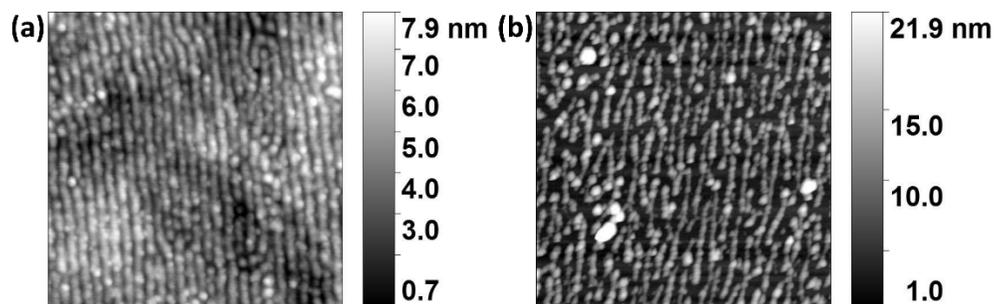
**Figure S1.** AFM height images of a shear-aligned and Pt-infiltrated PS-P2VP film **(a)** before and **(b)** after removal of the block copolymer – an illustrative example of how the true quality of the metal nanowires may not be apparent until after polymer removal. Images are of 1  $\mu\text{m}$  x 1  $\mu\text{m}$  areas.
