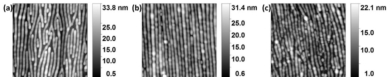
**Figure S6.** AFM height image showing the representative nanowire morphologies of 68.5-26 PS-P2VP that are (a) below the optimal shearing time (1 hr), resulting in poor alignment; (b) at the optimal shearing time (3 hrs), resulting in well aligned nanowires; and (c) above the optimal shearing time (4 hrs), resulting in a lower alignment quality. Images are of 1  $\mu\text{m}$  x 1  $\mu\text{m}$  areas.
