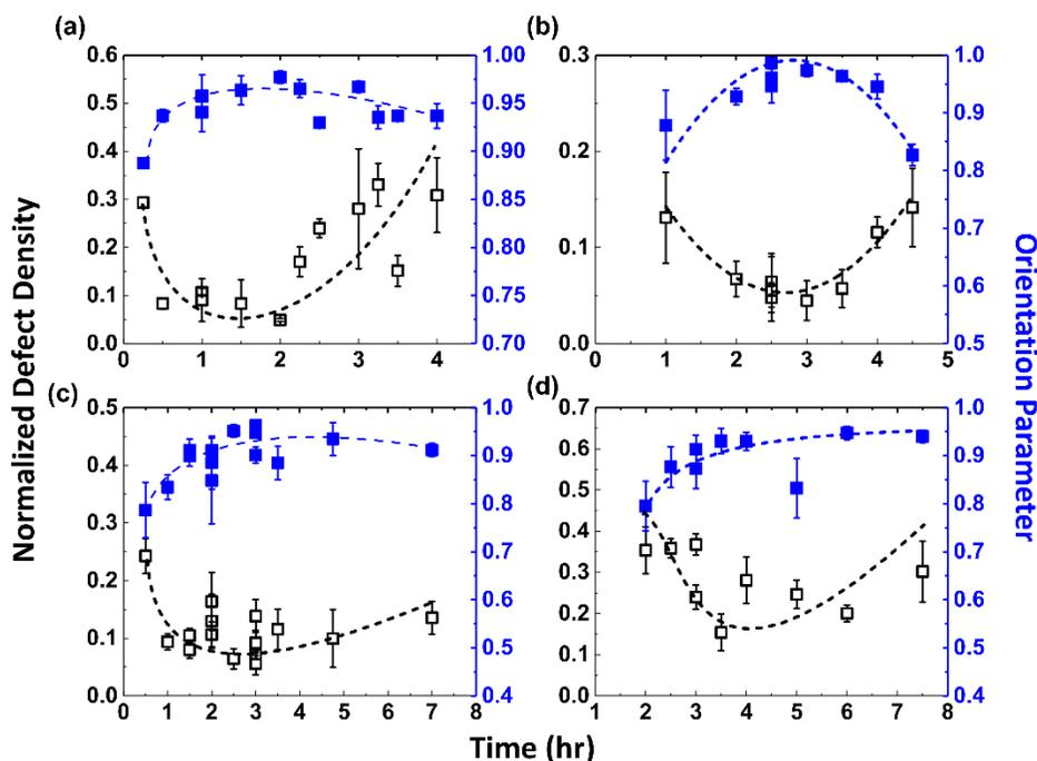
**Figure S5.** Normalized defect density (left axis, black open squares) and orientation parameter (right axis, blue filled squares) of nanowire arrays as a function of the duration of shear alignment for each molecular weight PS-P2VP: (a) 48-14, (b) 68-26, (c) 79-36, and (d) 110-52 kg/mol. Each data point represents a separate sample on which multiple measurements were made. Dashed lines are provided as a guide for the eye.
