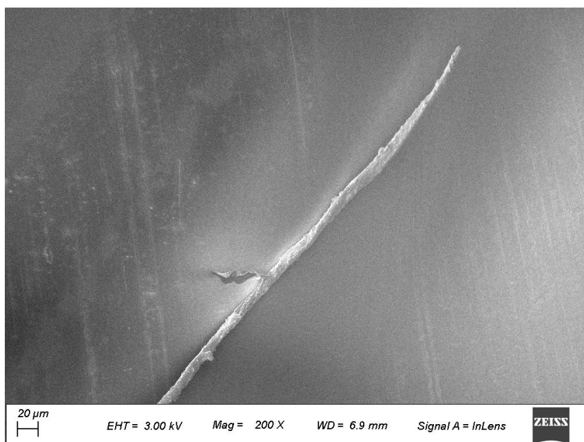
Fig. S25 FESEM image of co-aggregate of PNI and NH 2 -NMI in THF/ n -hexane ( v/v = 1:9). Image was captured after drop-casting a solution of co-aggregate, prepared by mixing PNI and NH 2 -NMI in 10:1 molar ratio.
