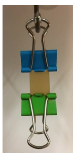
Figure S5 – Photograph of a typical repaired elastomer sample fixed between two clamps used for stress-rupture tests. To the lower clamp the respective weights with different masses were attached.
