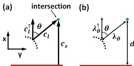
The above diagram shows this scenario expressed in terms of either (a) velocity or (b) distance. For a time period equal to  $t = \frac{d}{c_s} = \frac{\lambda_\theta}{c_l} = \frac{\lambda_\theta^\uparrow}{c_l^\uparrow}$ , the length of the (a) velocity vectors and (b) distances are equal. The value of  $c_l^\uparrow$  is given by
