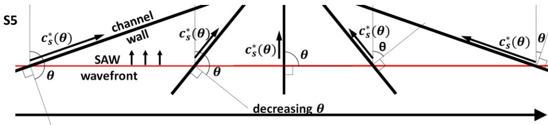
Noting that this effective  $c_s$  is a function of  $\theta$ , the intersection angle as a function of the channel wall angle is given by
