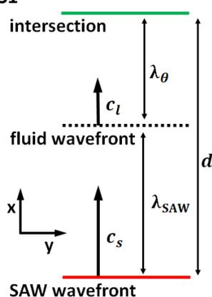
Looking at this in a simplified case where both wavefronts are travelling in the same direction, we can solve for  $\lambda_\theta$  with the knowledge that they intercept at time  $t$  from the initiation of the fluid wavelet.
