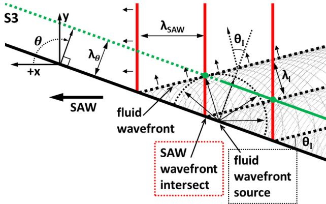
Because of this displacement, the time to fluid and SAW wavefront intersection (as described previously in Figure S1 and Equation S1) will change, and requires the consideration of a separate model to determine the value of  $\lambda_{\theta}$  for flat channel walls.
