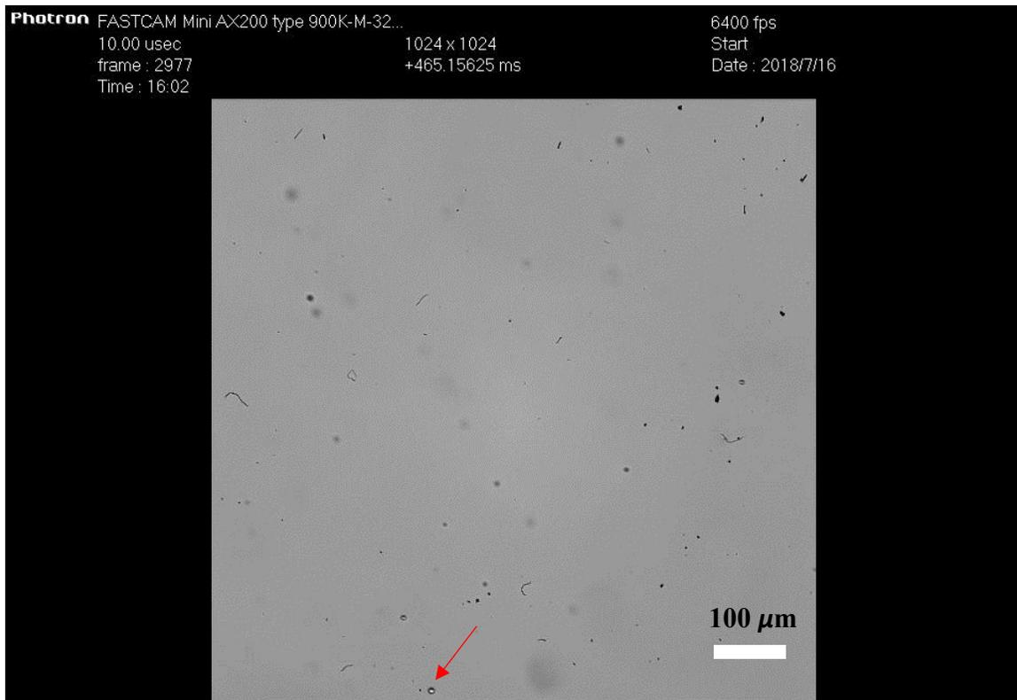
**Fig. S3.** Image of the fog particles captured by a high-speed camera (Photron Fastcam Mini AX200) at a frame rate of 6400 fps. Multiple images were taken and the average fog droplet radius was measured to be  $\sim 5 \mu\text{m} \pm 1 \mu\text{m}$ .
