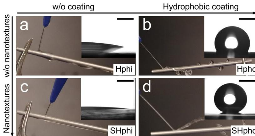
**Fig. S2.** Water droplet contact angles ( $\sim 5 \mu\text{L}$  in volume) and the behaviors of water flow that have been jetted onto (a) hydrophilic, (b) hydrophobic, (c) superhydrophilic, and (d) superhydrophobic wires. The wire diameter is 2.06 mm. Scale bars are 1 mm.
