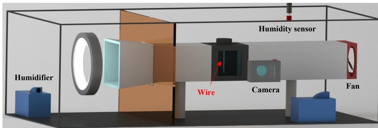
**Fig. S1.** Schematic of the experimental setup used in this study, including the environmental chamber, humidity sensor, wind tunnel, humidifiers, camera, and fan.
