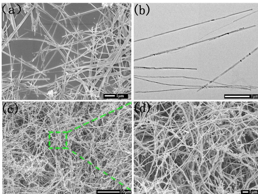
**Fig. S2** (a) FESEM image of HAPNWs; (b) TEM image of HAPNWs; (c) FESEM image of CNTs and (d) large magnification of (c).
