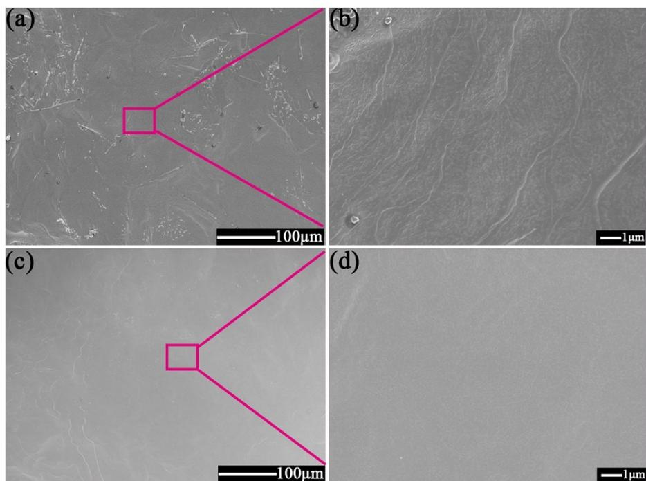
**Fig. S7** (a) and (c) represent the FESEM of PIHPHCF with the paraffin volume of 60 and 140 $\mu\text{l}/\text{cm}^2$ , respectively; (b) and (d) represent the large magnification of (a) and (c), respectively. Obviously, the more dosage of paraffin, the film surface will be more smoother.
