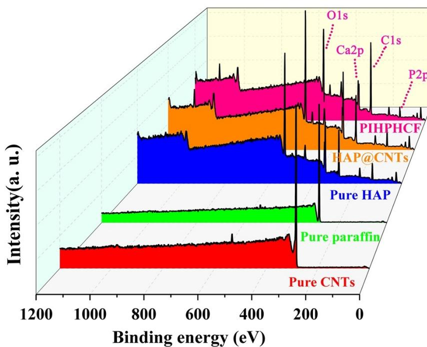
**Fig. S4** XPS spectra of pure CNTs, pure paraffin, pure HAPNWs, HAP@CNTs film and PIHPHCF, respectively.
