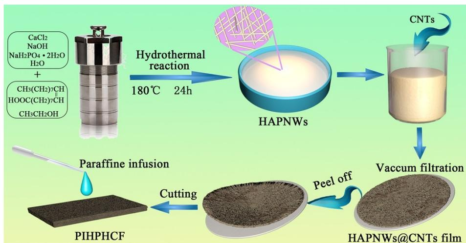
**Fig. S1** Schematic representation of the preparation procedure of PIHPHCF via the hydrothermal process and vacuum-assisted suction filtration.
