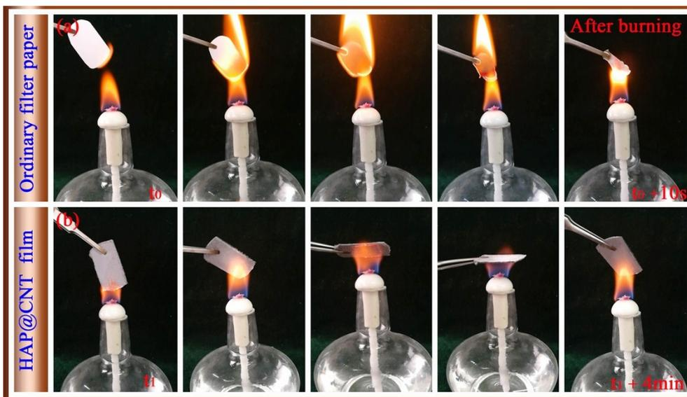
**Fig. S5** Thermal stability tests of (a) ordinary filter paper and (b) HAP@CNT film. Here, the HAP@CNT film shows excellent thermal resistance even it's exposed to fire for 4 minutes at 400-500°C. In the contrary, the ordinary filter paper severing as contrast experiments is burned to ashes within 10 seconds.
