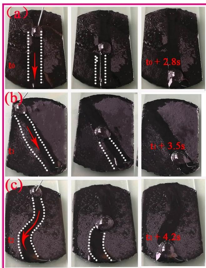
**Fig. S8** Optical photographs of NaOH liquid (PH=12, 20 $\mu\text{l}$ ) sliding on patterned slippery surface of
