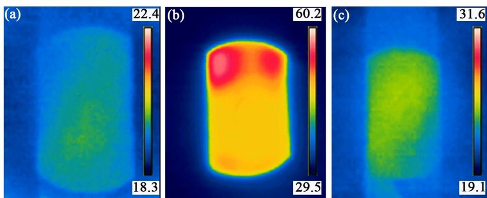
**Fig. S6** Infrared thermal image of PIHPHCF. (a) and (b) represent before and after the near-infrared light irradiation; (c) the melted surface cools to room temperature.
