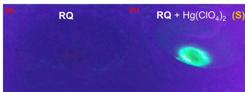
**Fig. S9.** Fluorescent responses of the (a) **RQ**, (b) **RQ + Hg(ClO<sub>4</sub>)<sub>2</sub>** solid sample.
