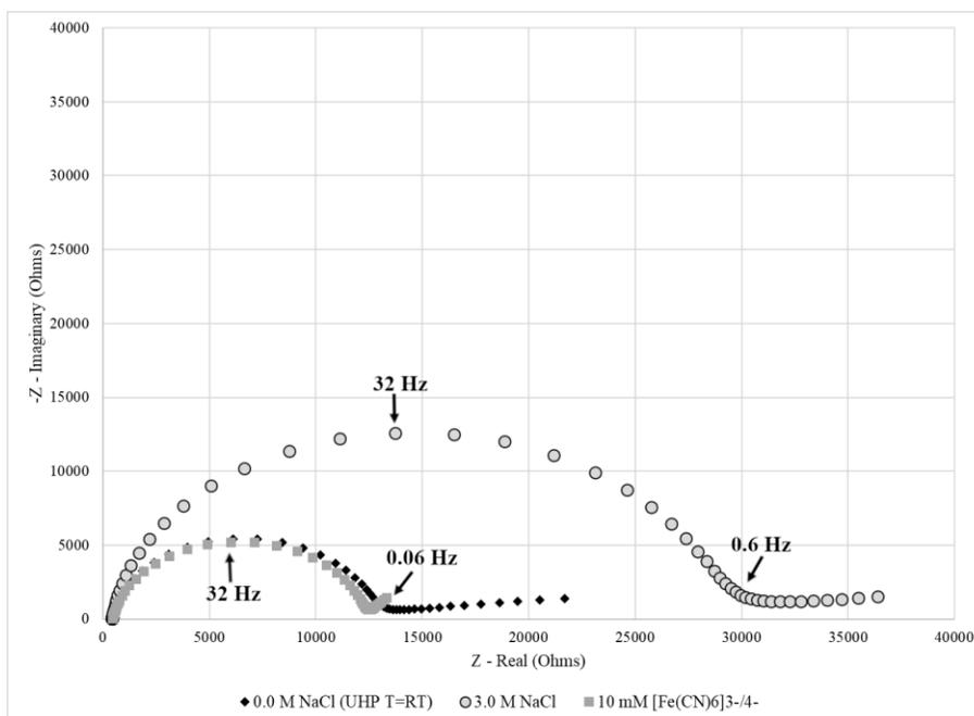
**Figure S5.** Impedance response obtained after soaking an I40 modified electrode in the redox couple solution
