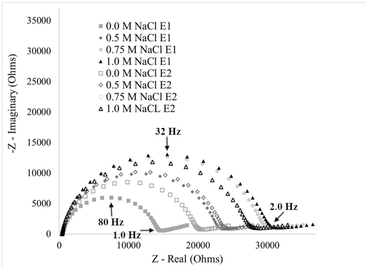
**Figure S6.** Replicate data of the impedance response from an I40 modified electrode after exposure to 0.0 M NaCl-1.0 M NaCl. An intermediate state between the maxima and minima is observed at both electrodes under a 0.5 M NaCl condition.
