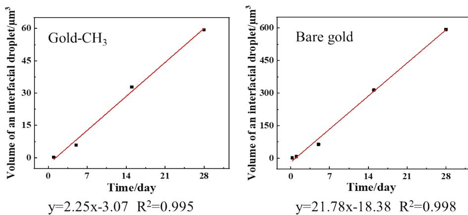
**Fig. S1** Volume of interfacial droplets on hydrophobic substrates (gold-CH<sub>3</sub> and bare gold) changes with time.
