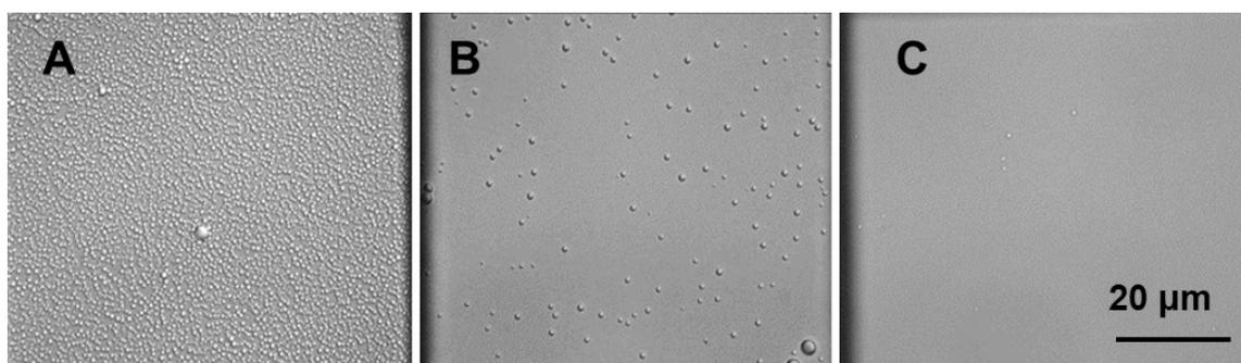
**Fig. S3** The interfacial droplets formed between n-hexadecane and monolayers formed from (A)  $\text{HS}(\text{CH}_2)_{11}\text{CH}_3$  (B)  $\text{HS}(\text{CH}_2)_{15}\text{CH}_3$  and (C)  $\text{HS}(\text{CH}_2)_{17}\text{CH}_3$  on gold, incubated in water for 5 days.
