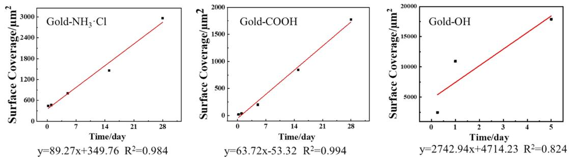
**Fig. S2** Surface coverage of interfacial droplets on hydrophilic substrates (gold-NH<sub>3</sub>·Cl, gold-COOH and gold-OH) changes with time.
