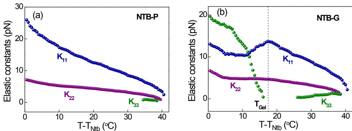
**Figure S5:** Comparison of the thermal dependence of all the three Frank elastic constants for the (a) NTB-P and (b) NTB-G mixtures.
