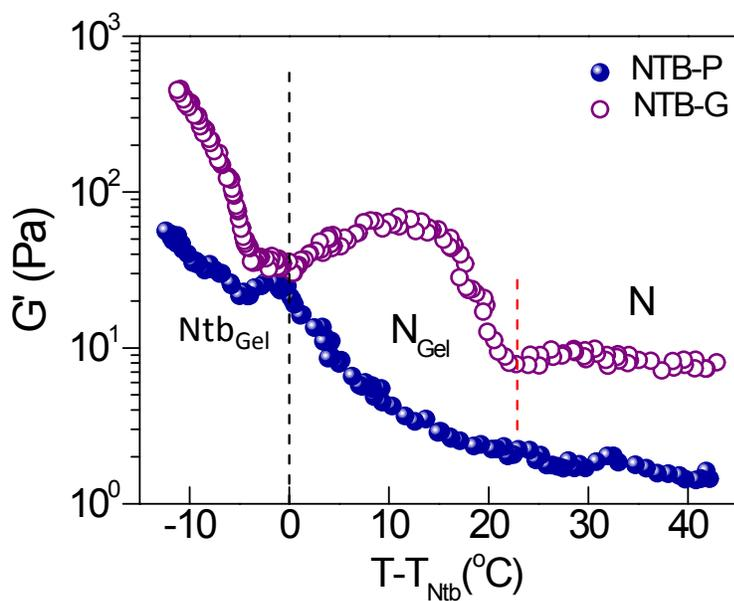
**Figure S2:** Temperature dependence of the storage modulus,  $G'$  of the NTB-P and NTB-G systems. The y-axis is in log scale. The vertical red dotted line demarcates the *N* (sol) phase from the  $N_{Gel}$  in the NTB-G mixture.
