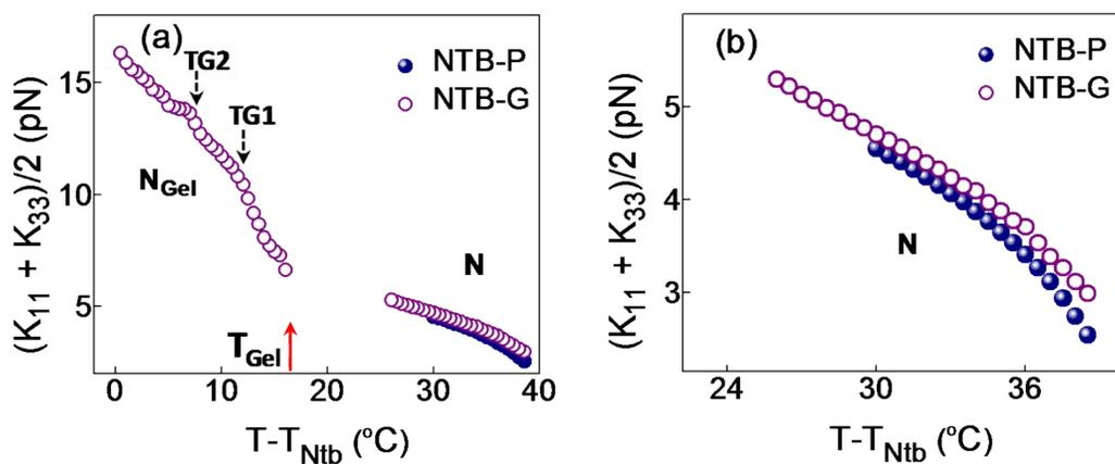
**Figure S6:** Thermal dependence of the average elastic constant,  $(K_{11} + K_{33})/2$  for the NTB-P and NTB-G mixtures (a) in the entire thermal range and (b) expanded view of the profiles in the nematic phase. The vertical red arrow in (a) demarcates the  $N$  (sol) phase from the  $N_{Gel}$  in the NTB-G mixture.
