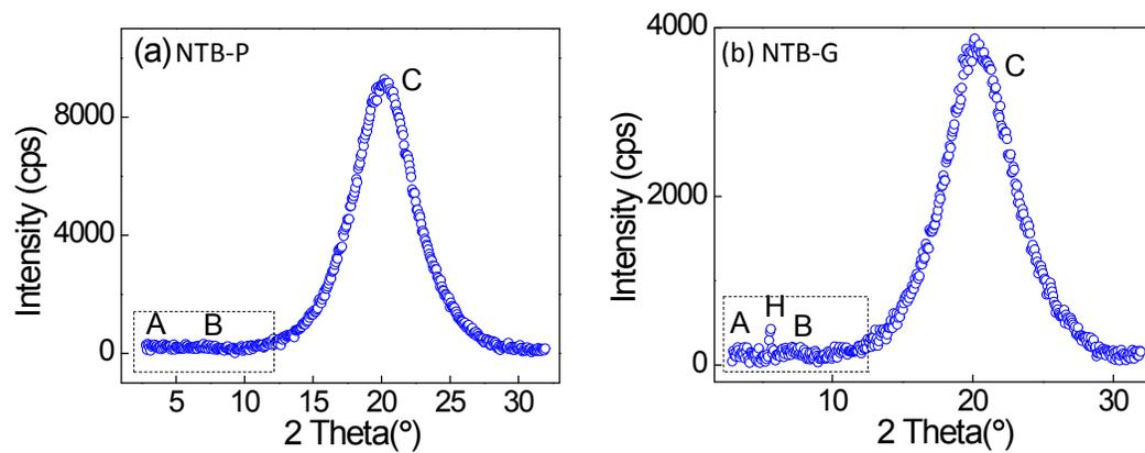
**Figure S7:** XRD profiles of (a) NTB-P and (b) NTB-G mixtures exhibiting the low angle peaks (shown inside the dotted rectangle) 'A', 'B' along with the HSA peak 'H' and the wide-angle peak 'C'
