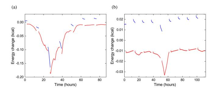
**Figure S1.** Raw data of time-resolved quasi-isothermal DSC measurements of two samples: (a) pure DLPE, (b) 90:10 DLPE:DLPG (mole %). The red curves are heating scans and the blue curves are cooling scans. There is a mismatch between cooling and heating scan data possibly due to the different scanning rates (see experimental section).
