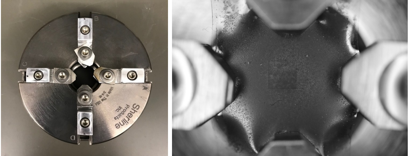
Figure S12: (left) The biaxial stretcher, composed of a lathe chuck equipped with toe clamps. (Right) a representative image of a sample used for DIC analysis.
