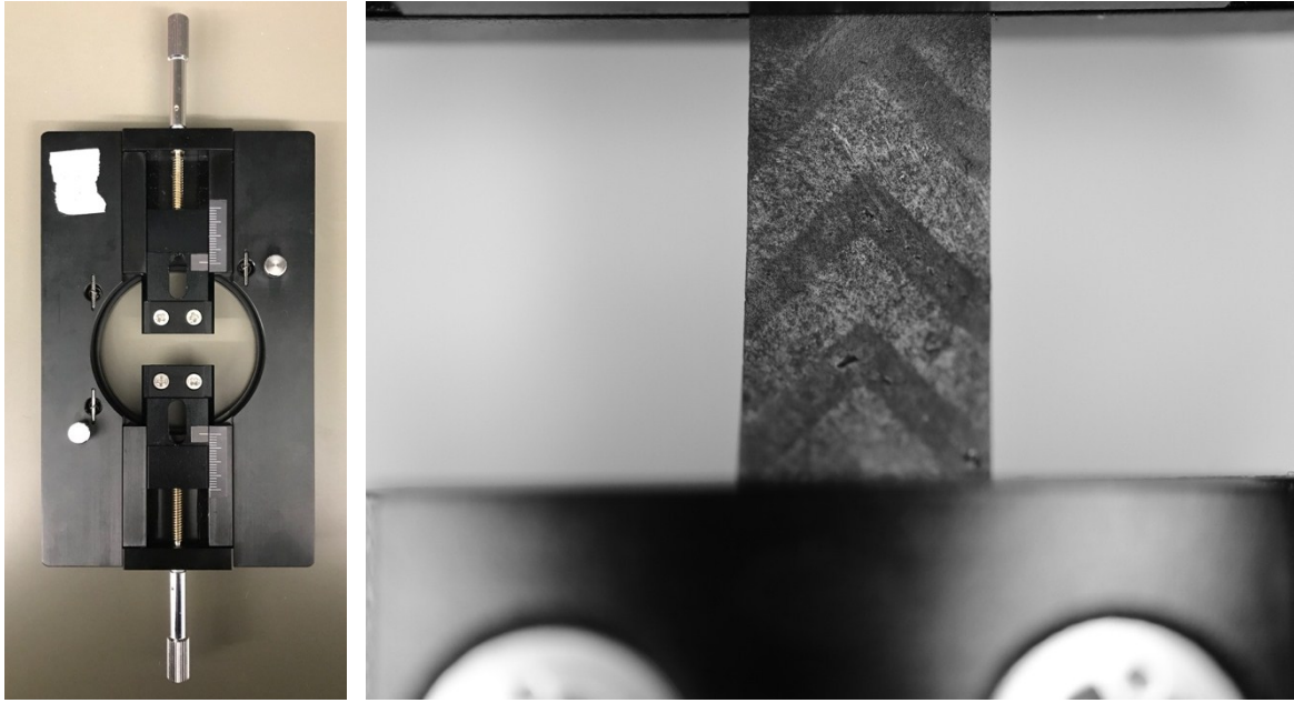
Figure S11: (left) The microvice tensile holder and (right) a representative image of a sample during DIC analysis.
