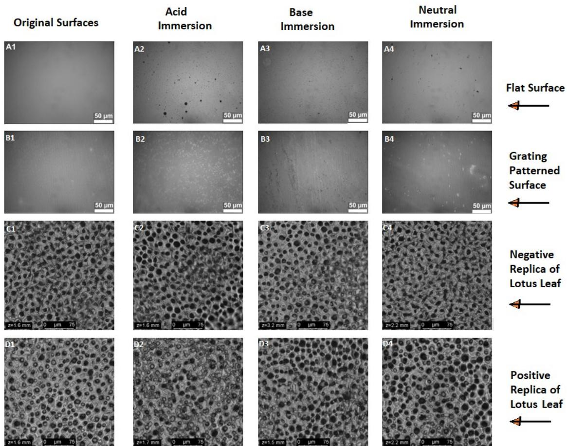
**Fig. S5.** Composite of microscope images after  $t_I = 7$  days. Each column represents the type of immersion medium and each row represents the type of the surface which are marked in the figure.
