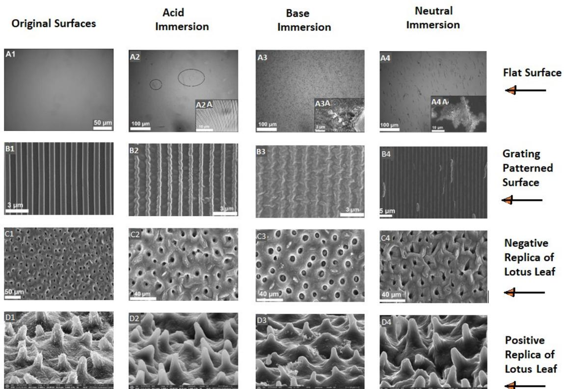
**Fig. S4.** Composite of microscope images after  $t_1 = 31$  days. Each column represents the type of immersion medium and each row represents the type of the surface which are marked in the figure.
