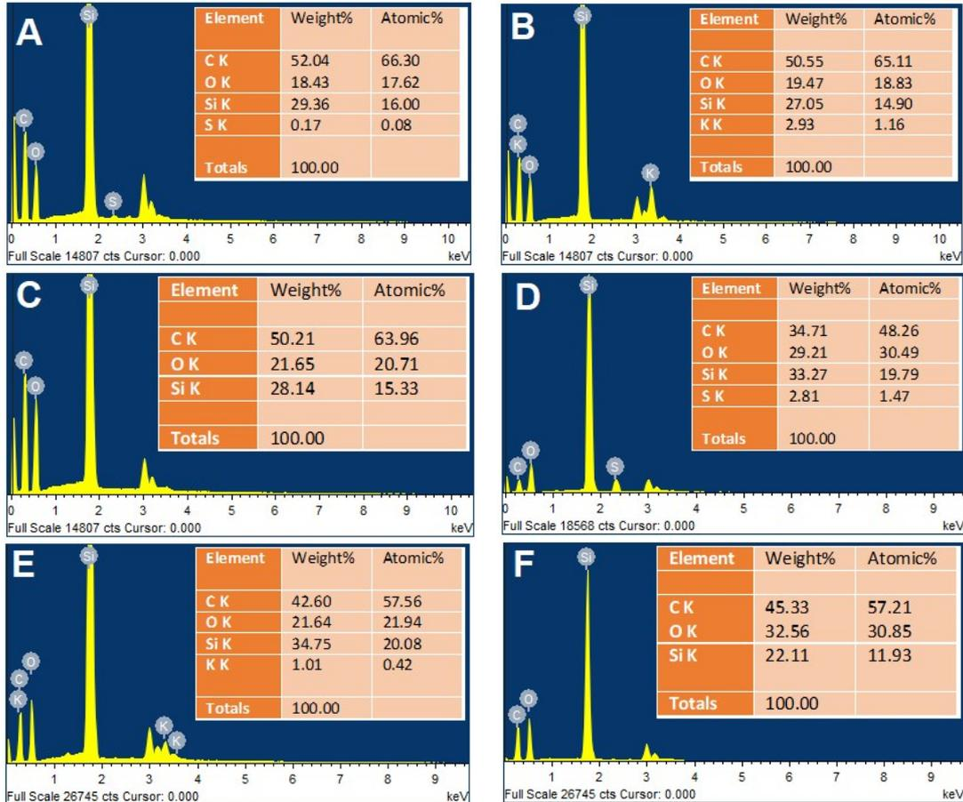
**Fig. S2** EDS analysis of negative and positive replicas of lotus leaf. Negative replicas immersed in (A) acidic, (B) basic, and (C) neutral solutions. The corresponding SEM images are shown as insets B1, D1 and F1 respectively in Fig. 4 of the main article. Positive replica of lotus leaf immersed in (D) acidic, (E) basic and (F) neutral mediums. The corresponding SEM images are shown as insets B1, D1 and F1 respectively in Fig. 5 of the main article.
