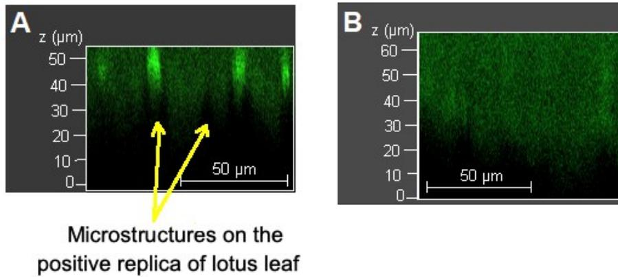
**Fig. S3** Confocal microscopy cross section image of biomimetic positive replica of lotus leaf immersed under water containing Rhodamine B dye: (A) After 10 mins of immersion showing partially penetration of the liquid meniscus and entrapped air pockets, and (B) at same position after 1 hr of immersion. The images show that the water penetrates gradually in between the surface asperities.
