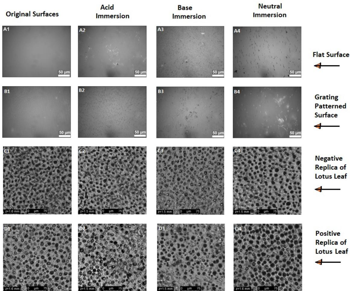
**Fig. S6.** Composite of microscope images after  $t_1 = 18$  days. Each column represents the type of immersion medium and each row represents the type of the surface which are marked in the figure.
