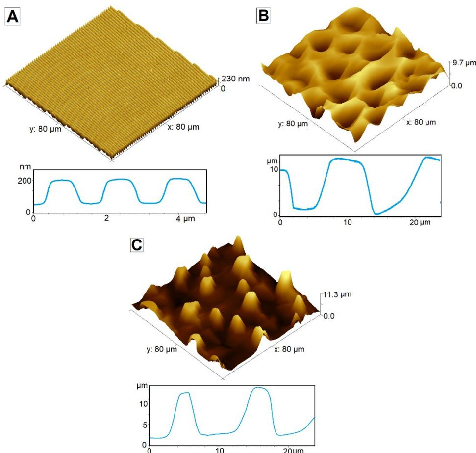
**Fig. S1** AFM images of the patterned Sylgard 184 samples along with cross sectional profiles. (A) Grating patterned sample with feature height ( $h_p$ ) = 230 nm and periodicity ( $\lambda_p$ ) = 1.5 μm. (B) Biomimetic negative replica of lotus leaf with average hole depth ( $h_D$ ) = 9.7 μm and average hole diameter ( $d_H$ ) = 5.9 μm. (C) Biomimetic positive replica of lotus leaf with average pillar height ( $h_p$ ) = 11.3 μm and average pillar diameter ( $d_p$ ) = 4.2 μm.
