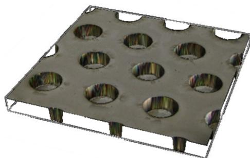
**Fig. S10** Laser scanning confocal microscope image of the micropatterned mold made by acryl resin. The diameter and height of the cylindrical holes is 91 and 96  $\mu\text{m}$ , respectively.
