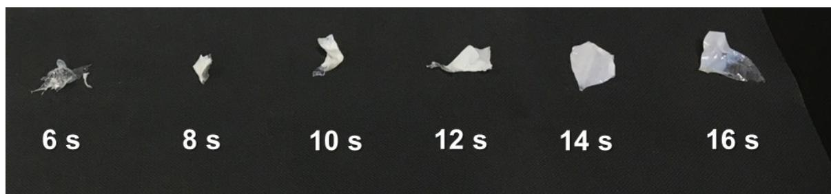
**Fig. S5** Photographs of partially crosslinked polydomain LCEs after extracted with  $CHCl_3$  for 48 h, followed by vacuum drying. Each LCE were prepared by UV crosslinking with different exposure time as indicated in the image.
