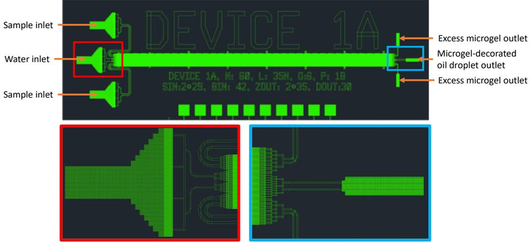
FIG. S7: The DLD device has a mirrored design to allow for greater sample throughput.
