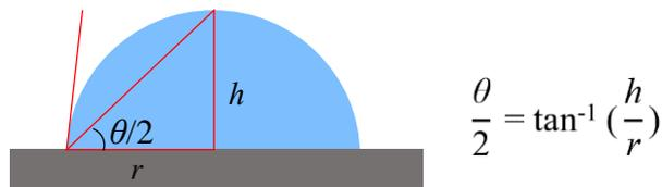
**Fig. s7** Schematic of contact angle measurement by  $\theta/2$  method
