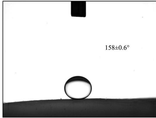
**Figure S10.** The optical image of a oil droplet (3  $\mu\text{L}$ ) with a contact angle of  $158\pm 0.6^\circ$  on the surface of the APNC gel underwater.
