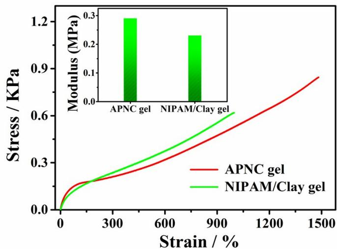
**Figure S4.** Tensile strength and modulus of the APNC gel (0.85 MPa, 0.29 MPa) and the NIPAM/Clay gel (0.62 MPa, 0.23 MPa).
