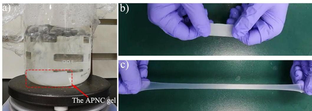
**Figure S5.** a) The process of the APNC gel keeping in boiling seawater. b&c) The illustrations of the excellent mechanical properties of the APNC gel after keeping in boiling seawater for 30 min.
