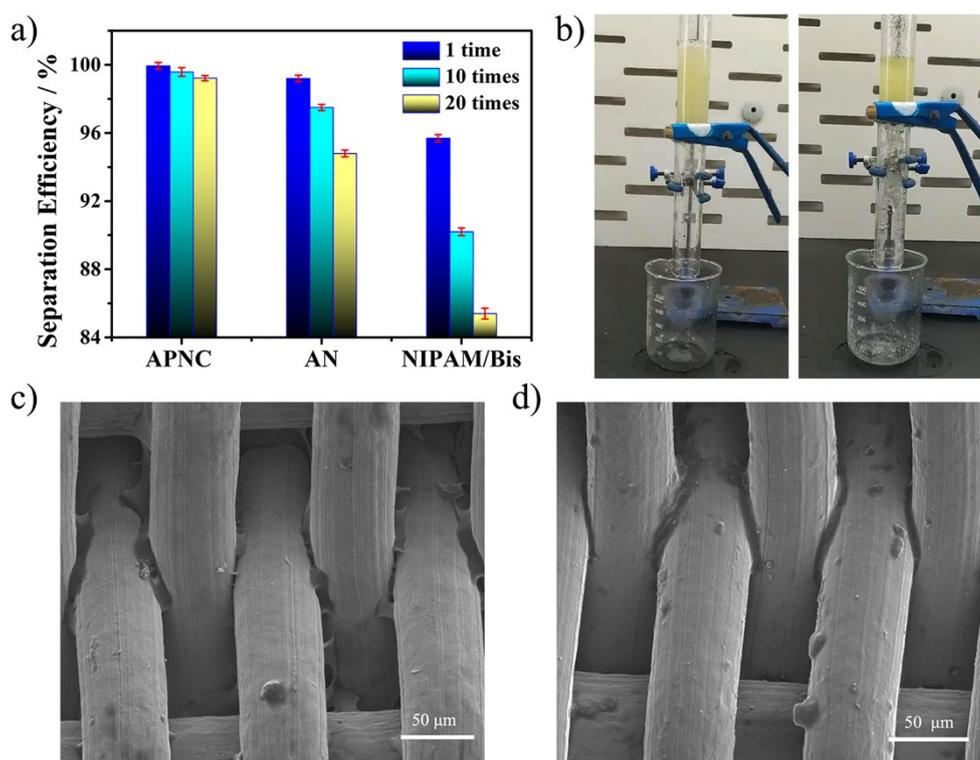
**Figure S13.** a) The separation efficiencies of the different gel-coated mesh (APNC gel, AN gel and NIPAM/Bis gel). The oil was vegetable oil and the oil content was 50 v/v%. b) The process of the oil/seawater separation by the NIPAM/Bis gel-coated mesh. c&d) The SEM images of the AN gel-coated mesh (c) and NIPAM/Bis gel-coated mesh (d), and the mesh is 300.
