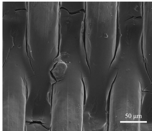
**Figure S11.** The SEM images of the APNC gel-coated stainless steel mesh.
