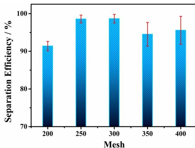
**Figure S12.** The separation efficiency of the gel coated mesh with different pore size, including 200 (74  $\mu\text{m}$ ), 250 (61  $\mu\text{m}$ ), 300 (50  $\mu\text{m}$ ), 350 (43  $\mu\text{m}$ ), 400 (38  $\mu\text{m}$ ) mesh.
