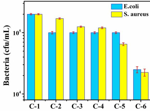
**Figure S8.** The counts of the bacteria (*E. coli* and *S. aureus*) attaching to APNC gel with different clay content (C-n: hydrogel containing 0.05n g/mL clay) after being maintained for 72 h.
