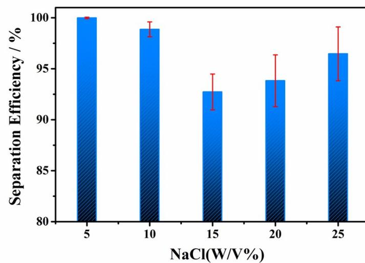
**Figure S14.** The separation efficiency of oil/water mixtures of diesel oil and seawater with different NaCl concentration (5-25 wt%).
