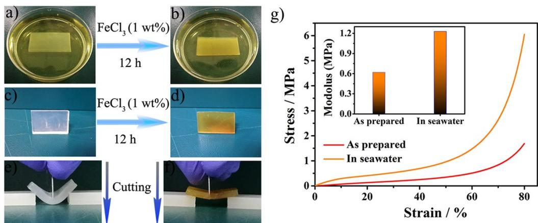
**Figure S6.** a-d) The images of the APNC gel before (a&c, transparent) and after (b&d, brown) immersed in FeCl<sub>3</sub> solution for 12 hours. e&f) The cutting process of the as prepared APNC gel (e) and the Fe<sup>3+</sup> enhancement APNC gel (f) with the same cutting force and speed. g) The compressive strength and modulus of the as-prepared APNC gel (1.68 MPa, 0.62 MPa) and the APNC gel immersed in FeCl<sub>3</sub> solution for 12 h (6.05 MPa, 1.23 MPa).
