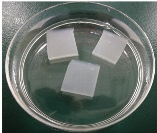
**Figure S7.** The image of the APNC gel after immersed in seawater for more than 1 month.
