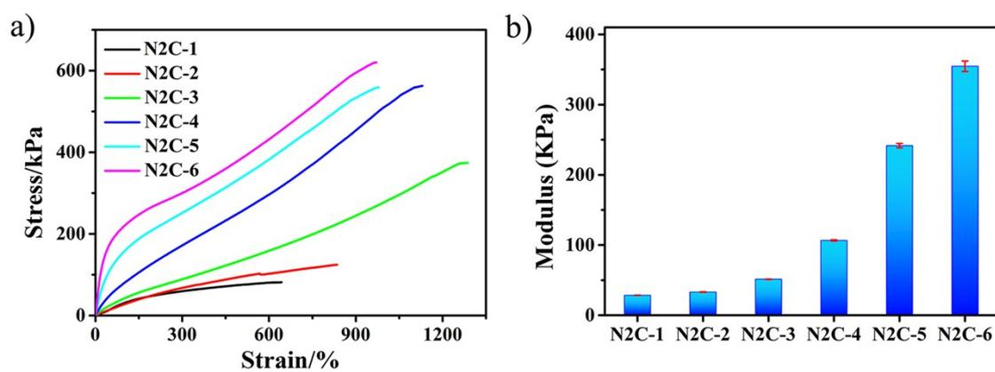
**Figure S3.** a) Stress-strain curves of the APNC gels with different clay contents (N2C-n: hydrogel containing 0.05n g/mL clay). The concentration of agar was 0.01g/mL, and NIPAM was 0.1g/mL. b) The modulus of the as-prepared APNC gel with different clay contents.
