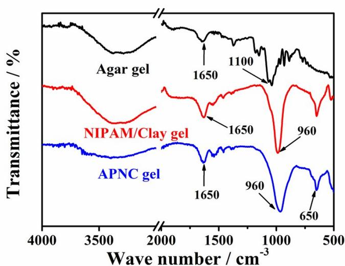
**Figure S1.** FT-IR spectra of Agar, NIPAM/Clay, and APNC gels. The peaks at 1650 cm<sup>-1</sup> and 1100 cm<sup>-1</sup> were contributed to N-H bending and O-H stretching vibration, respectively, 960 cm<sup>-1</sup> and 650 cm<sup>-1</sup> were the absorption peaks for Si-O stretching and metallic oxide stretching (Li-O, Mg-O, etc.), respectively.
