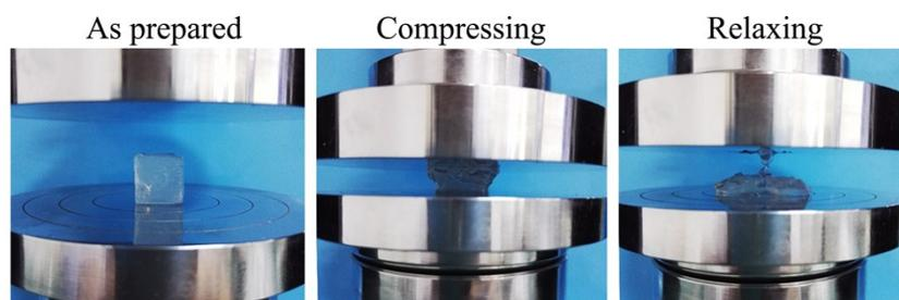
**Figure S2.** The compression tests of the agar gel.
