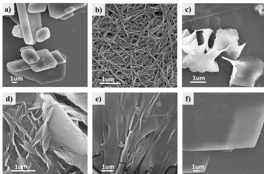
**Figure S2.** SEM images of Nap-2 in a) THF, b) THF: H<sub>2</sub>O=1:2, volume ratio, c) THF: H<sub>2</sub>O=1:4, volume ratio, d) THF: H<sub>2</sub>O=1:6, volume ratio, e) THF: H<sub>2</sub>O=1:8, volume ratio, f) H<sub>2</sub>O.
