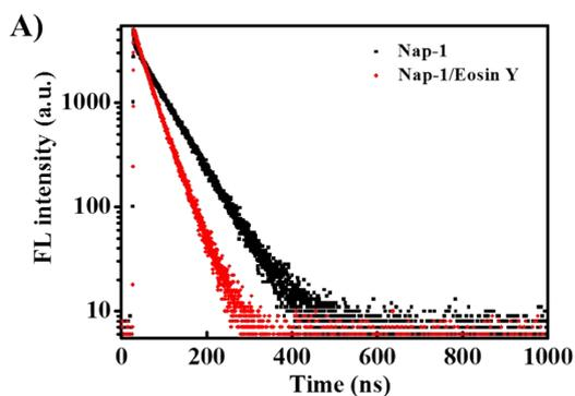
**Figure S8.** Time-resolved emission of Nap-1 and Nap-1/20% Eosin Y co-assembly, semilogarithmic scale, detected at 320 nm.  $\lambda_{ex} = 260$  nm.
