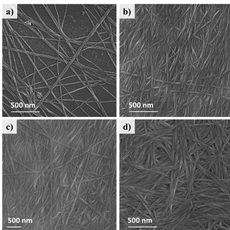
**Figure S6.** The SEM image of Nap-1 and Eosin Y co-assemblies in THF/H<sub>2</sub>O mixed solution. a) The SEM image of Nap-1. b), c) and d) The SEM image of Nap-2 was co-assembled with 5%, 10%, 20% Eosin Y, respectively.
