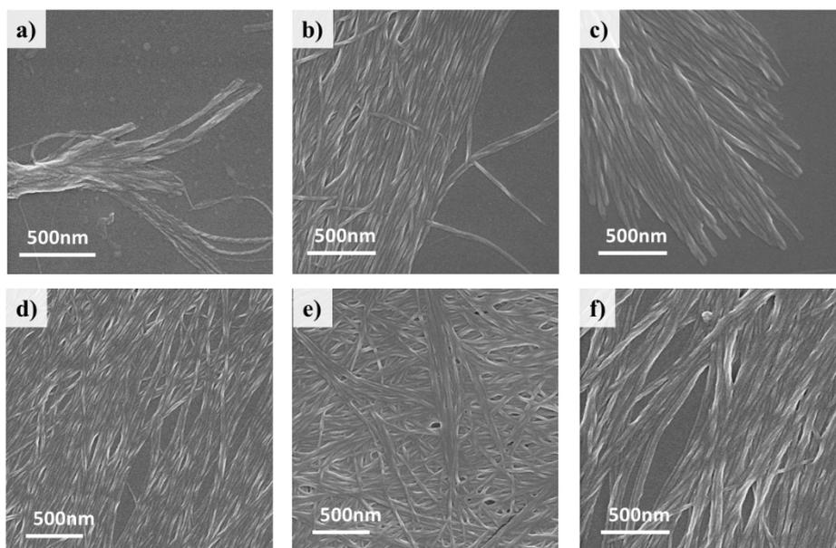
**Figure S1.** SEM images of Nap-1 in a) THF, b) THF: H<sub>2</sub>O=1:2, volume ratio, c) THF: H<sub>2</sub>O=1:4, volume ratio, d) THF: H<sub>2</sub>O=1:6, volume ratio, e) THF: H<sub>2</sub>O=1:8, volume ratio, f) H<sub>2</sub>O.
