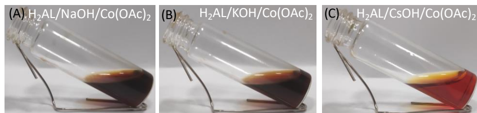
Figure S1. The gelation test of gelator 1 with (A) \text{Na}^+ , (B) \text{K}^+ , (C) \text{Cs}^+ .
