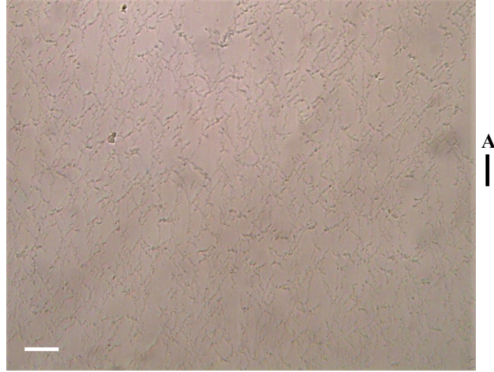
Fig S3. Optical texture of [CCN-mn (0.75)] taken in a planar cell with only the analyzer when the fibrous strands within the BFDs are revealed. Scale bar corresponds to 50 \mu\text{m} .
