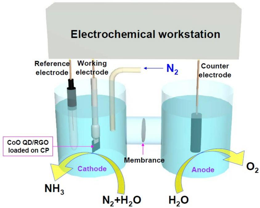
Fig. S8. Schematic of H-type electrochemical setup.
