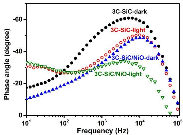
**Figure S7.** (A) Bode phase plots of 3C-SiC and 3C-SiC/NiO in the dark or under AM1.5G 100 mW/cm<sup>2</sup> illumination.
