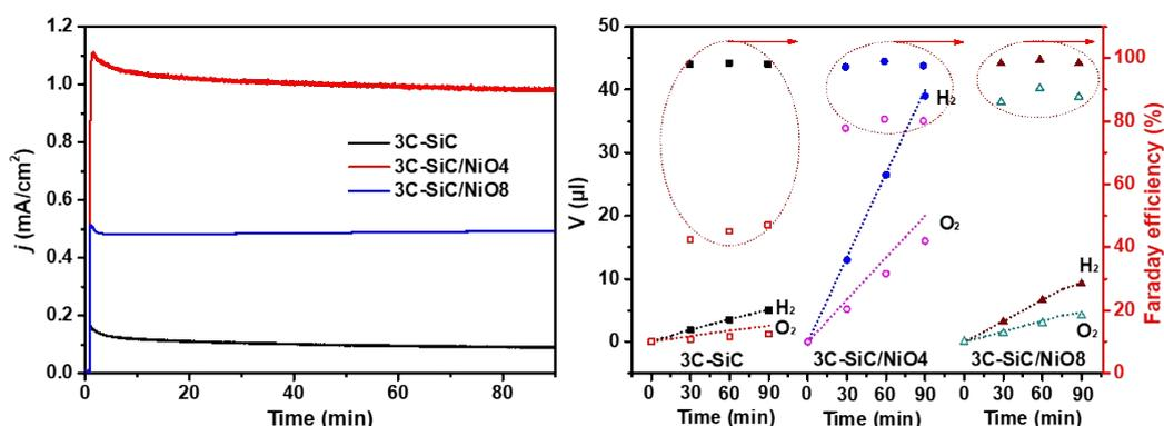
**Figure S5.** The photocurrent densities (A) and the  $H_2$  and  $O_2$  Faradaic efficiencies (B) of the 3C-SiC and 3C-SiC/NiO-4min, and 3C-SiC/NiO-8min photoanodes at  $1.0 V_{RHE}$  under steady-state AM1.5G  $100 \text{ mW/cm}^2$  illumination in  $1.0 \text{ M NaOH}$  solution. Faradaic efficiencies of the evolved  $H_2$  and  $O_2$  were obtained from gas chromatography measurement.
