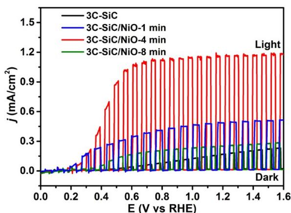
**Figure S3.** Current density-potential curves of the 3C-SiC and 3C-SiC/NiO photoanodes with NiO deposition for 1, 4, 8 minutes in 1.0 M NaOH under chopped AM1.5G 100 mW/cm<sup>2</sup> illumination, at the scan rate of 30 mV/s.
