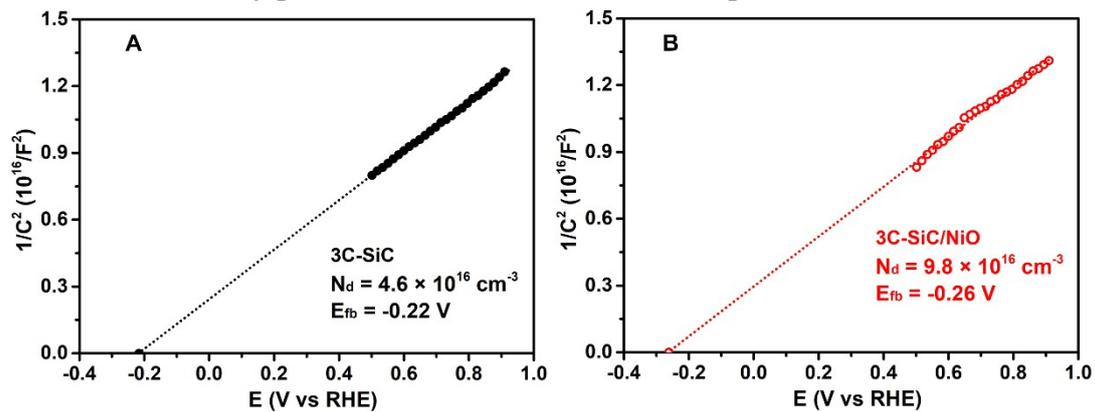
**Figure S6.** Mott-Schottky plots of 3C-SiC and 3C-SiC/NiO-4min photoanodes in 1.0 M NaOH solution. The flat-band potentials were obtained from the intercepts of the extrapolated lines and the doping concentrations were calculated from the slopes.
