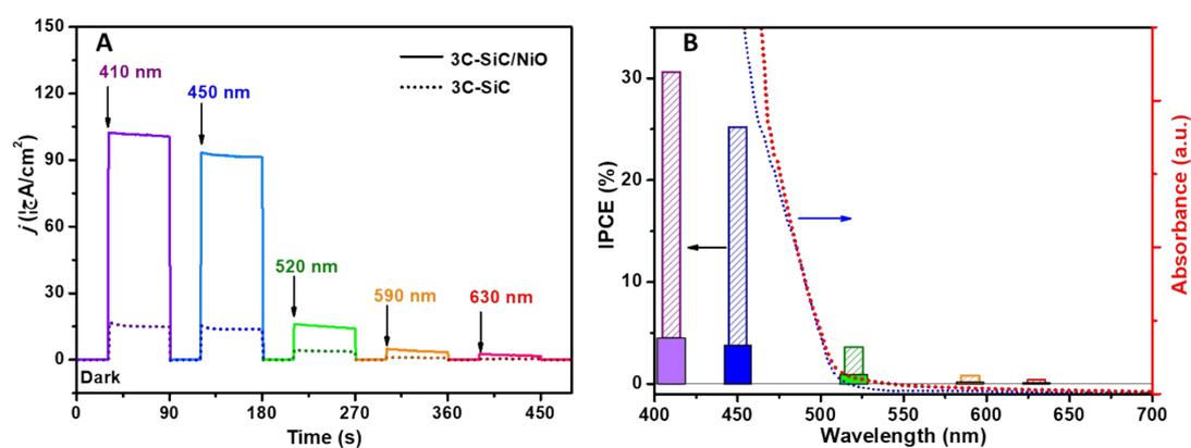
**Figure S4.** J-V curves (A) and the IPCE (B) of 3C-SiC/NiO-4min photoanode measured in 1.0 M NaOH solution at a bias of 1.0  $V_{\text{RHE}}$ , with scan rate of 30 mV/s. The different wavelength LEDs (line width of  $\sim 10$  nm) with a light power of 1 mW/cm<sup>2</sup> were used as light sources.
