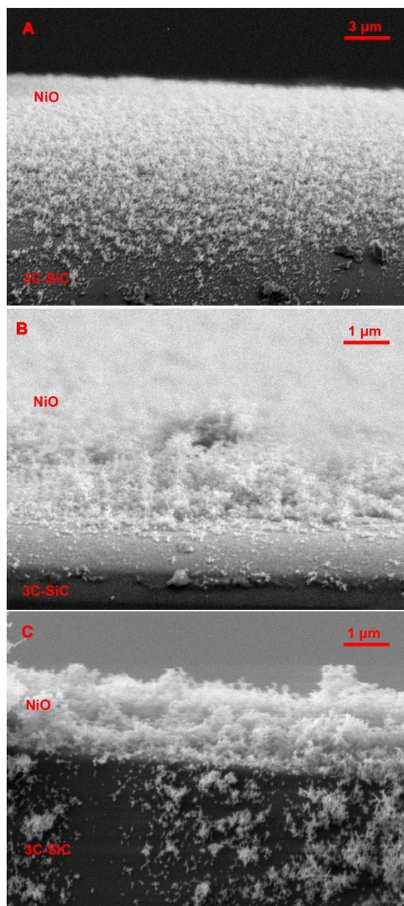
**Figure S1.** Side-view SEM images of 3C-SiC samples with NiO deposition for 1 min (A), 4 min (B) and 8 min (C).
