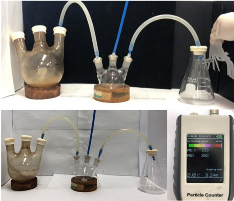
Fig. S3 Images showing delivery of PM-laden polluted air from left source chamber to right detection chambers by air flow.
