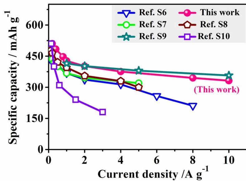
**Fig. S10.** Rate behavior of MoS<sub>2</sub>-based anodes for SIBs from previous literatures compared against the current work.
