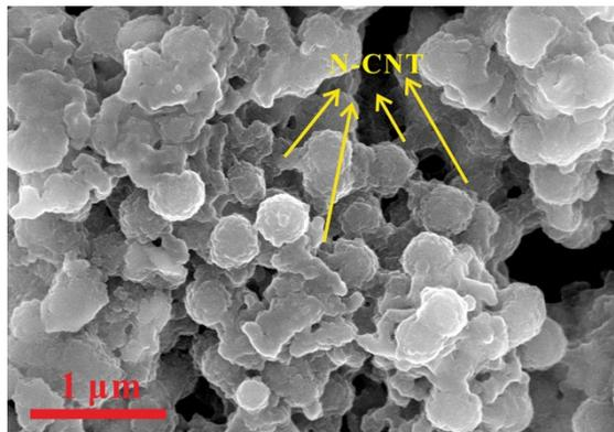
**Fig. S6.** SEM of MoS<sub>2</sub>/N-CNT electrode after 800 cycles at a current density of 2 A g<sup>-1</sup> for LIBs.
