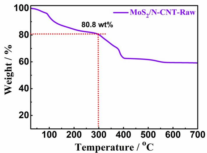
**Fig. S4.** TG curve of MoS<sub>2</sub>/N-CNT-Raw composite from room temperature to 700 °C under air.
