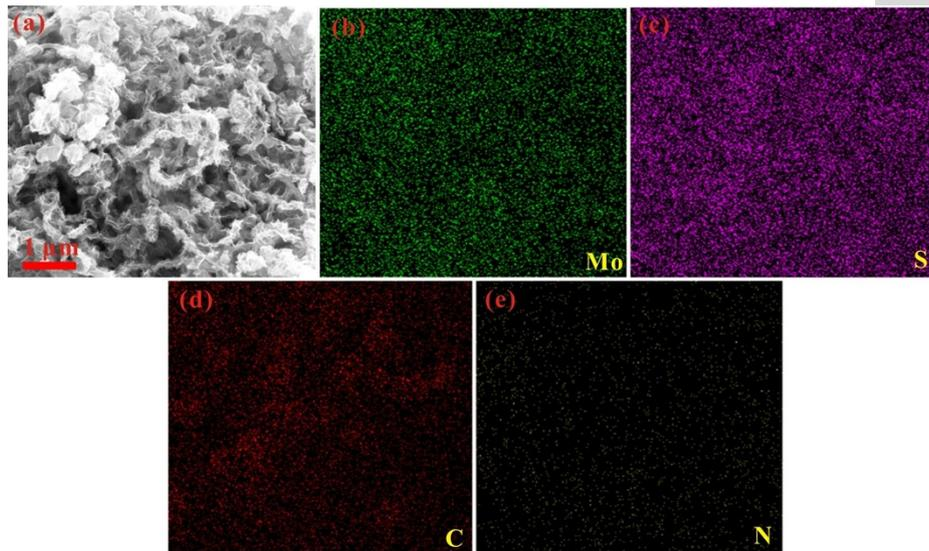
**Fig. S2.** The SEM (a) and elemental mapping images (b-e) of MoS<sub>2</sub>/N-CNT.
