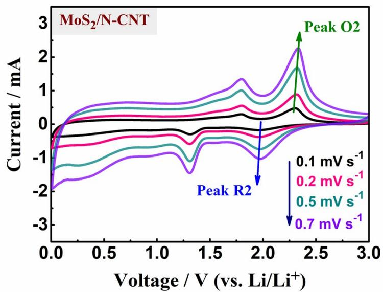
**Fig. S8.** CV curves of MoS<sub>2</sub>/N-CNT electrode at various scan rates from 0.1 mV s<sup>-1</sup> to 0.7 mV s<sup>-1</sup>.
