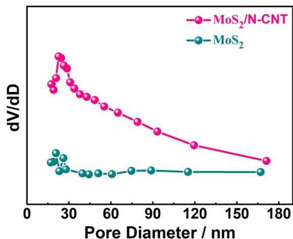
**Fig. S3.** The pore size distribution results of MoS<sub>2</sub> and MoS<sub>2</sub>/N-CNT based on their adsorption curves.
