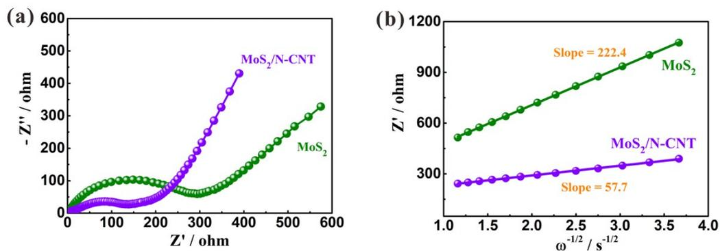
**Fig. S9.** (a) Nyquist plots of pure MoS<sub>2</sub> and MoS<sub>2</sub>/N-CNT composite after 100 cycles at 200 mA g<sup>-1</sup> for SIBs. (b)  $Z'$  vs  $\omega^{-1/2}$  plots of MoS<sub>2</sub> and MoS<sub>2</sub>/N-CNT for Warburg impedance analysis.
