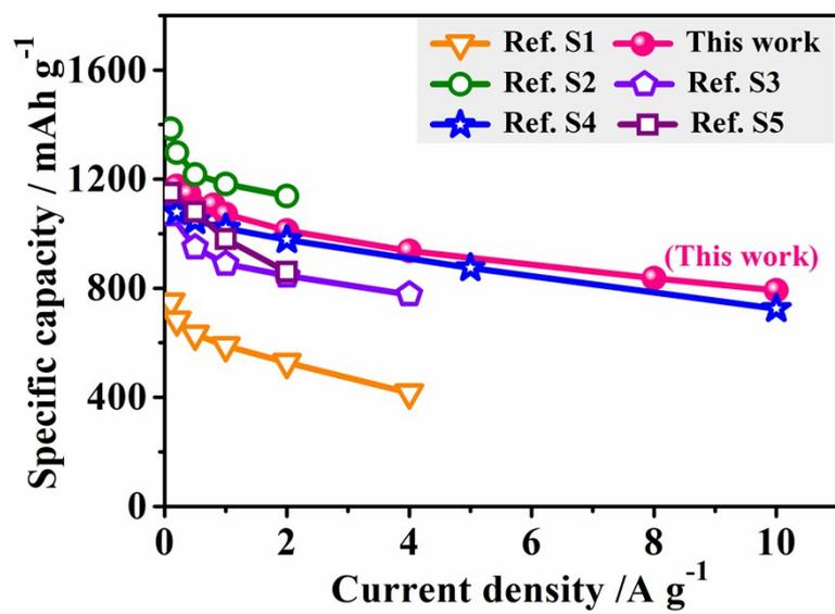
**Fig. S7.** Rate behavior of MoS<sub>2</sub>-based anodes for LIBs from previous literatures compared against the current work.
