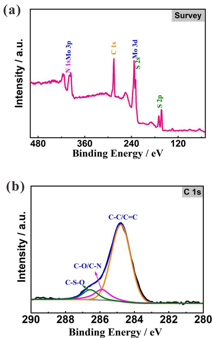
**Fig. S5.** (a) The survey spectrum of MoS<sub>2</sub>/N-CNT composite. (b) C 1s XPS spectrum of MoS<sub>2</sub>/N-CNT composite.
