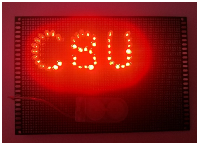
Figure S2 The successful light up of LED lamp bank with four aqueous Zn/Cu 3 (OH) 2 V 2 O 7 ·2H 2 O coin-cells.
