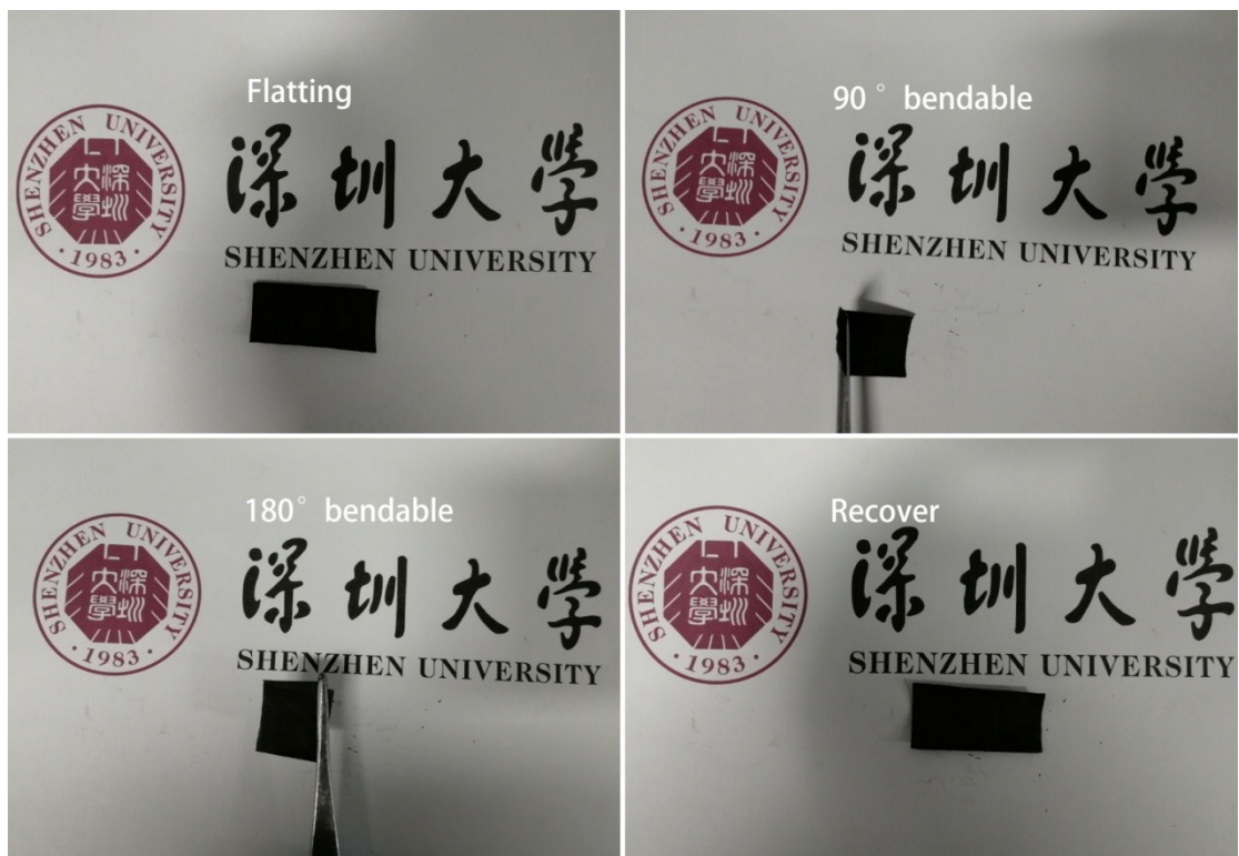
Fig S2. Digital images of PNCNF film under flattening, bending (90°, 180°) and recovered states.
