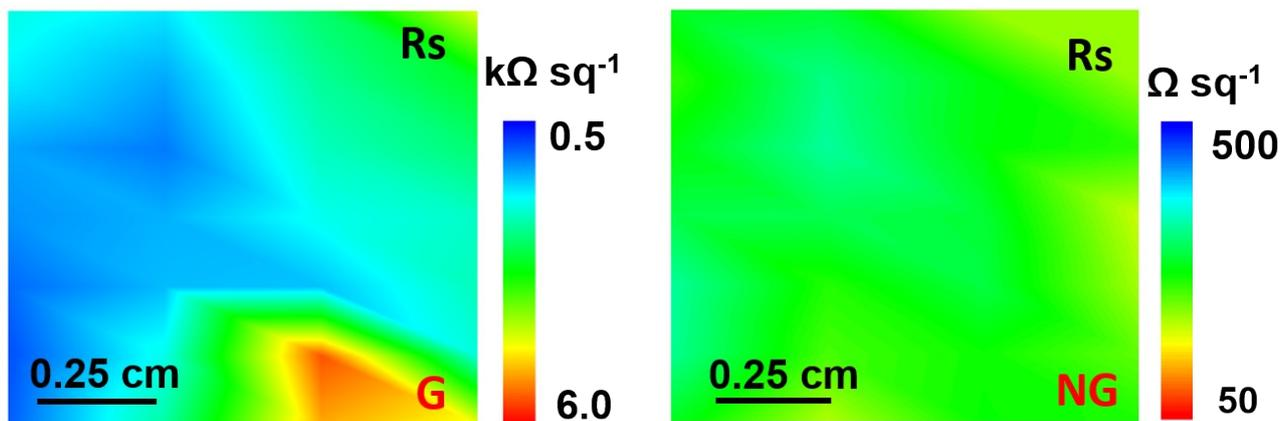
**Figure S16.** Spatial distribution of the sheet resistance of graphene and N-doped graphene film grown on flexible glass fiber cloth substrates.
