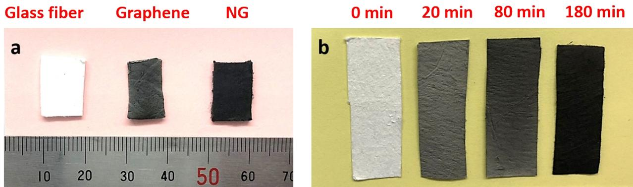
**Figure S14.** (a) Photograph of the pure flexible glass fiber cloth (left), graphene glass fiber cloth (center), and N-doped graphene glass fiber. (b) Photograph of as-grown flexible graphene glass fiber cloth samples obtained from different growth durations, with a bare glass fiber cloth (leftmost) displayed for comparison.
