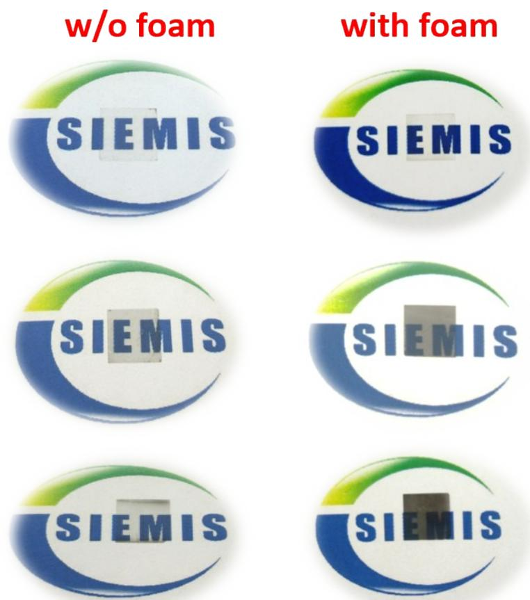
**Figure S9.** Photograph of mica-based graphene glass grown via PECVD without (left column) and with (right column) the copper foam assistance. The growth conditions for each row were kept identical (700 °C; 100 sccm Ar, 30 sccm H<sub>2</sub>, 10 sccm CH<sub>4</sub>; growth duration of 60 min, 120 min, and 180 min).
