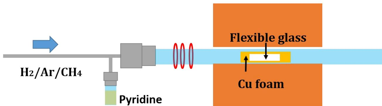
**Figure S12.** Schematic set-up of PECVD apparatus for the growth of N-doped graphene glass.
