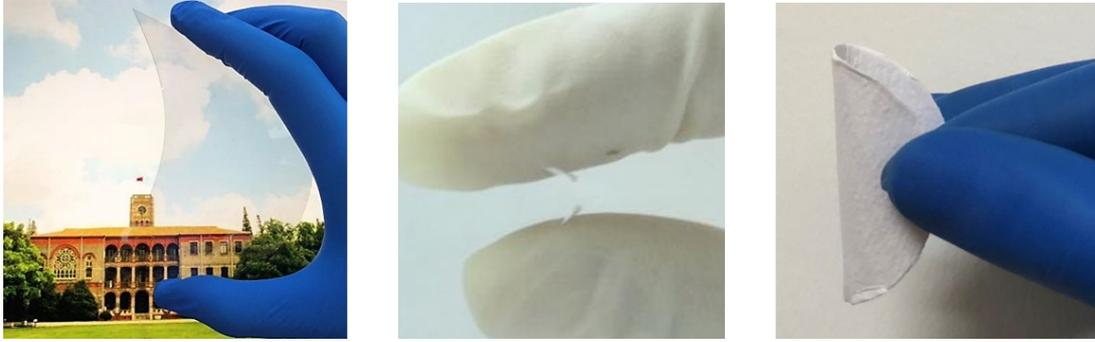
**Figure S1.** Photograph of the pristine flexible substrates (from left to right): flexible glass, mica sheet, glass fiber cloth.
