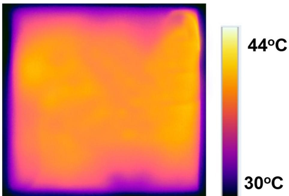
**Figure S10.** Surface temperature mapping of flexible graphene glass (10 cm × 10 cm) upon light exposure for 100 s.
