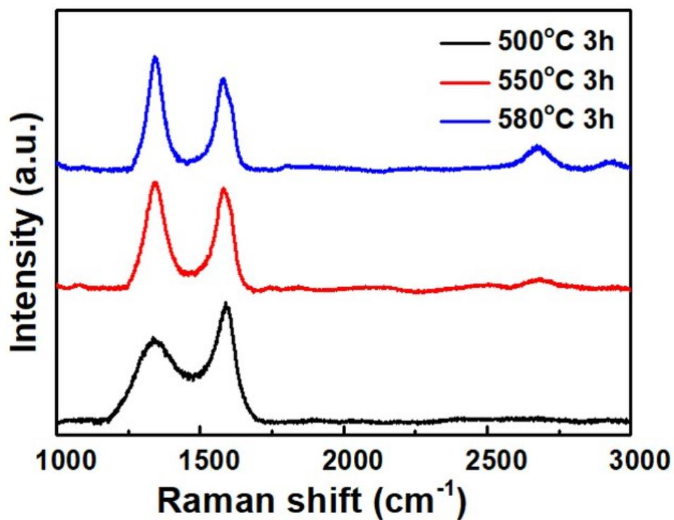
**Figure S15.** Representative Raman spectra obtained from flexible N-doped glass fiber cloth samples grown at 500 °C, 550 °C, and 580 °C, respectively.
