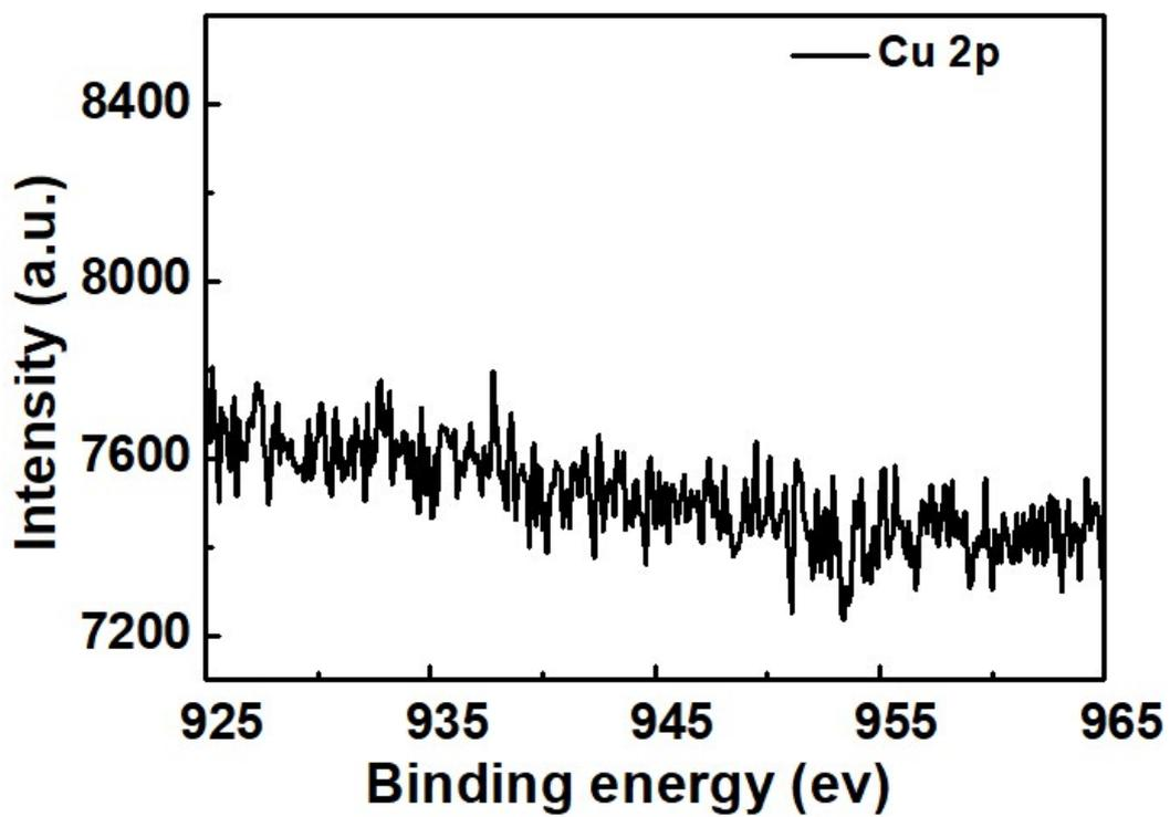
**Figure S3.** XPS Cu 2p spectrum of as-produced graphene glass after copper-foam-assisted PECVD reaction, showing the absence of Cu species.
