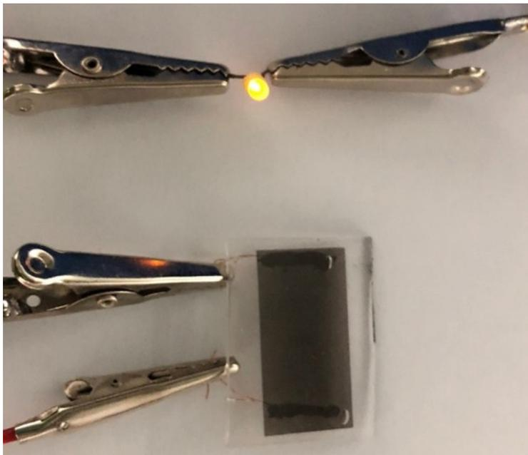
**Figure S11.** Direct integration of as-produced flexible graphene glass as a conductive electrode (flat state) toward lighting up the LED indicator.
