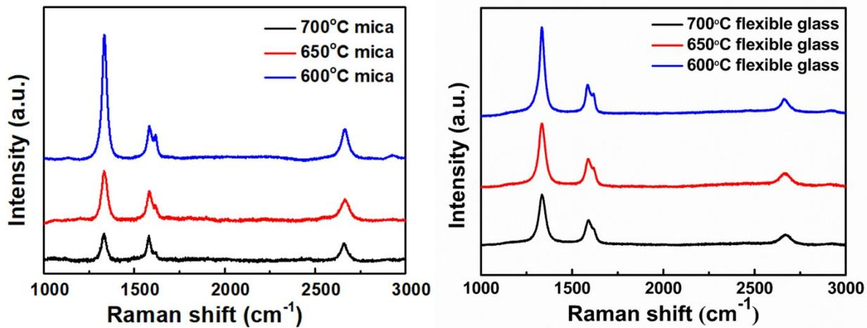
**Figure S6.** Raman spectra of graphene directly grown on mica and flexible glass substrates under different growth temperatures.
