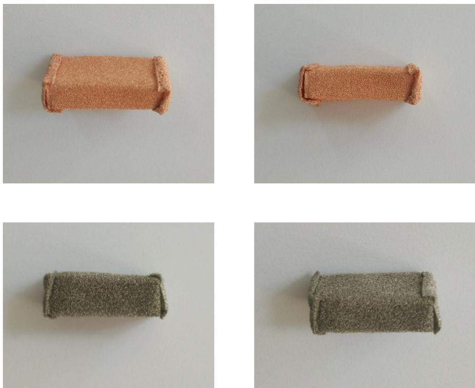
**Figure S2.** Photograph of typical copper-foam-cage and nickel-foam-cage with the size of 4 cm (length)  $\times$  2 cm (width)  $\times$  1 cm (height).
