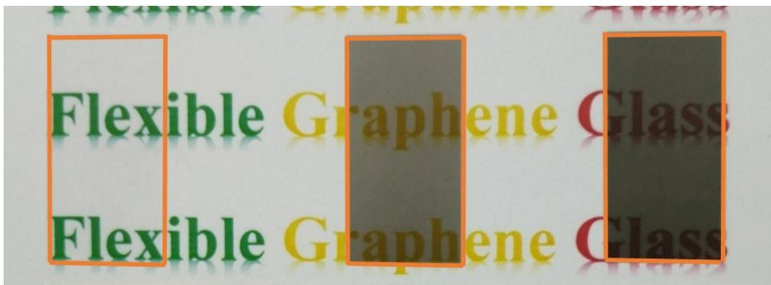
**Figure S13.** Photograph of as-grown N-doped graphene glass samples ( $3.0 \text{ cm} \times 1.5 \text{ cm}$ ) obtained for growth time of 60 min and 120 min with a bare flexible glass substrate (leftmost) shown for comparison.
