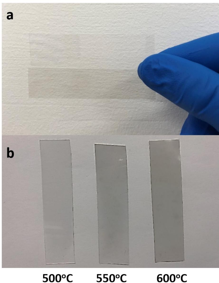
**Figure S5.** (a) Photograph of the as-grown flexible graphene glass (lower sample) exhibiting good uniformity as compared to bare substrate (upper sample). (b) Photograph of as-grown flexible graphene glass samples (1 cm × 5 cm) obtained at a growth temperature of 500 °C, 550 °C, and 600 °C, respectively (Growth condition: Ar:H<sub>2</sub>:CH<sub>4</sub> at a flow rate of 100:30:10 sccm, growth duration of 60 min, radio frequency at 80 W).
