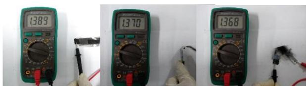
Figure S27 Photograph of all-flexible-solid-state rechargeable Zn-air battery with open circuit voltage at different angle
