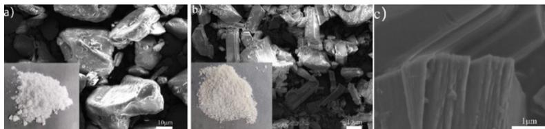
Figure S1 SEM images of melamine (a) before hydrothermal process and (b, c) after hydrothermal process; the insets are digital photograph respectively
