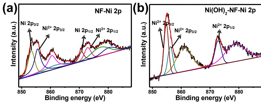
**Figure S5.** (a-b) The X-ray photoelectron spectroscopy (XPS) spectra of Ni foam,  $\text{Ni(OH)}_2$ .
