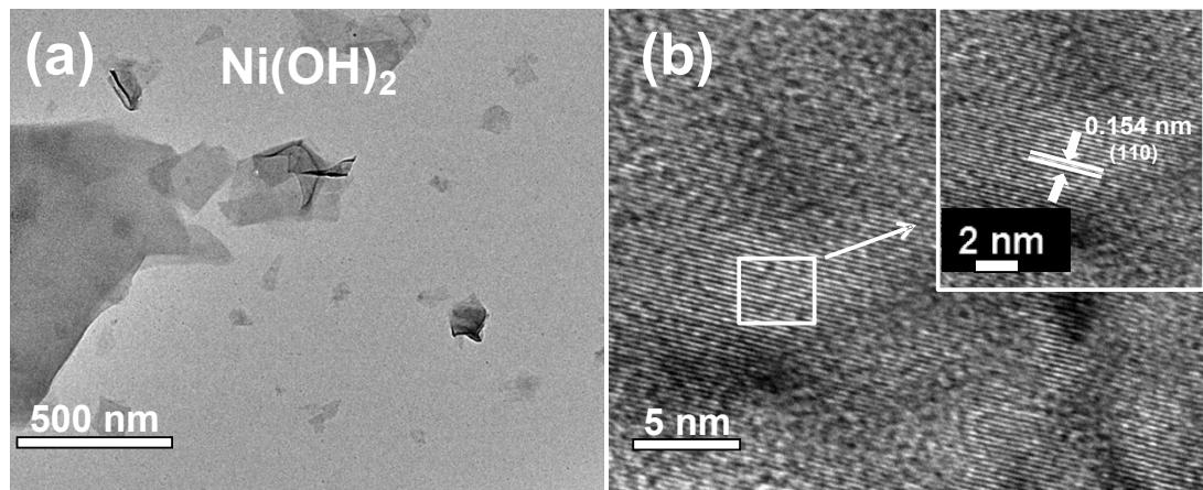
**Figure S6.** (a-b) The TEM and HRTEM of the  $\text{Ni(OH)}_2$ , the high resolution (HR) TEM image illustrates the lattice fringe space of 0.154 nm relating to the  $\text{Ni(OH)}_2$  (110).
