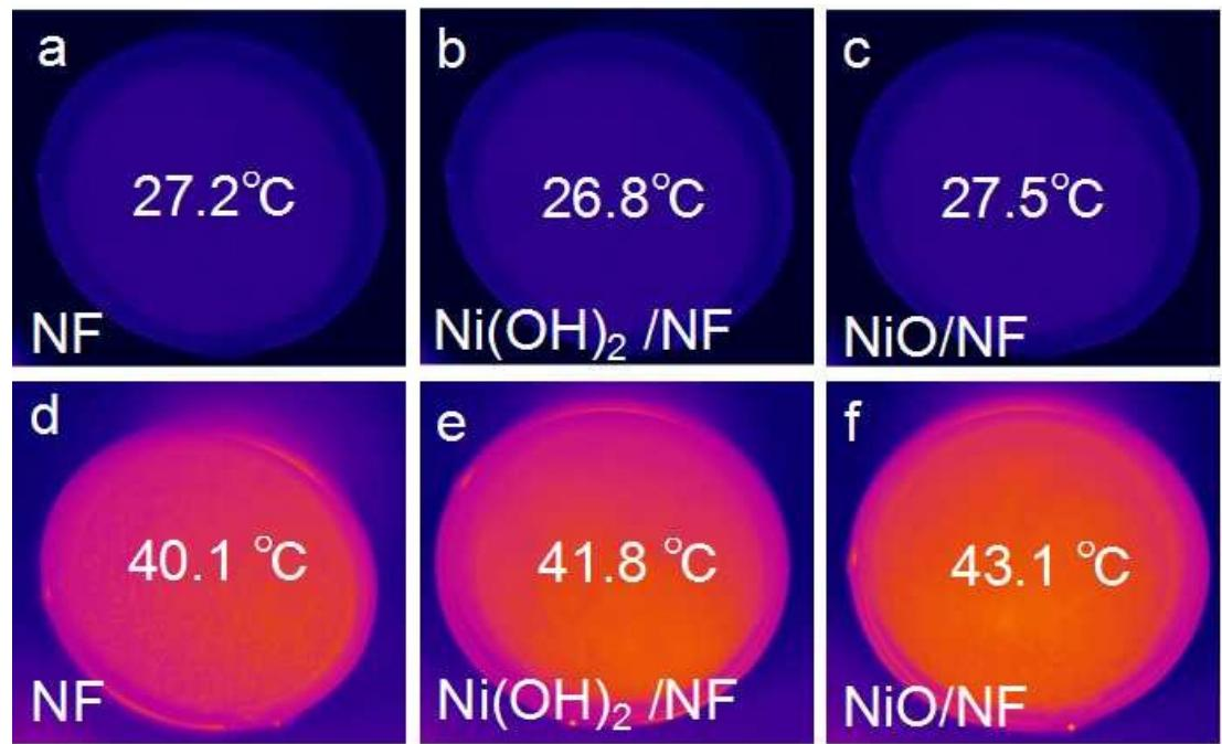
**Figure S9.** (a-f) The infrared images of water and NF, Ni(OH)<sub>2</sub>/NF and NiO/NF films floating on the water before and after 2 hours irradiation.
