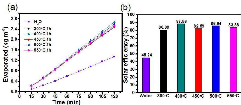
**Figure S10.** (a) The step 2 of the synthesis process (optimize preparation condition 1) : the dependence of evaporation rate of water on irradiation time for the different calcination temperature of  $\text{Ni(OH)}_2/\text{NF}$  samples under 1 sun simulated light ( $100 \text{ mW cm}^2$ ). The evaporation of water makes a blank contrast. (b) Corresponding solar efficiency of the above 6 samples.
