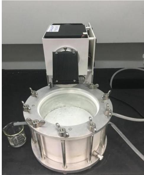
**Figure S1.** A home-made solar seawater desalination system to simulate solar seawater desalination.
