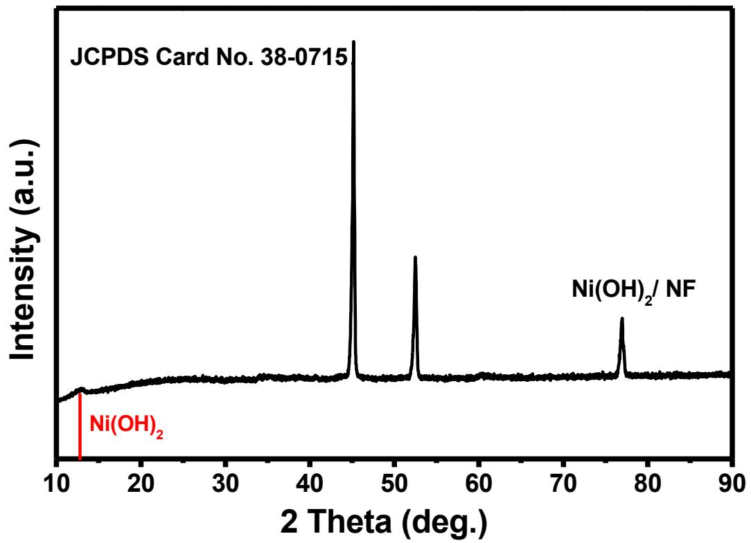
**Figure S2.** The X-ray diffraction (XRD) pattern of the Ni(OH)<sub>2</sub>/NF, JCPDS Card No.38-0715.
