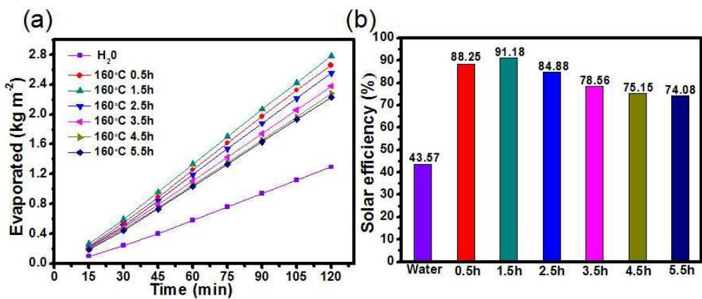
**Figure S12.** (a) The step 3 of the synthesis process (optimize preparation condition 3) : the dependence of evaporation rate of water on irradiation time for the different reduction time of NiO/NF samples under 1 sun simulated light (100 mW cm<sup>2</sup>). The evaporation of water makes a blank contrast. (b) Corresponding solar efficiency of the above 7 samples.
