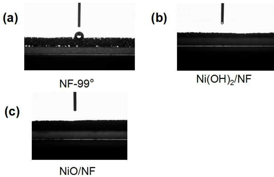
**Figure S8.** (a-c) The contact angles of the original Ni foam, Ni(OH)<sub>2</sub> nanosheets, NiO nanosheets samples display super hydrophilic behavior.
