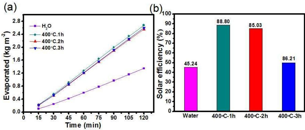
**Figure S11.** (a) The step 2 of the synthesis process (optimize preparation condition 2) : the dependence of evaporation rate of water on irradiation time for the different calcination time of Ni(OH)<sub>2</sub>/NF samples under 1 sun simulated light (100 mW cm<sup>2</sup>). The evaporation of water makes a blank contrast. (b) Corresponding solar efficiency of the above 4 samples.
