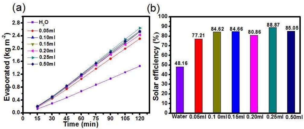
**Figure S13.** (a) The step 3 (Optimize preparation condition 4): the dependence of evaporation rate of water on irradiation time for the different reduction concentration of NiO/NF samples under 1 sun simulated light ( $100 \text{ mW cm}^2$ ). The evaporation of water makes a blank contrast. (b) Corresponding solar efficiency of the above 7 samples.
