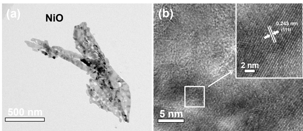
**Figure S7.** (a-b) The TEM and HRTEM of the  $\text{Ni}(\text{OH})_2$ , the high resolution (HR) TEM image illustrates the lattice fringe space of 0.243 nm relating to the  $\text{NiO}(111)$ .
