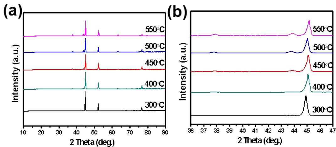
**Figure S4.** (a) The X-ray diffraction (XRD) pattern of NiO/NF at different temperature being reduced. (b) Intensity variation diagram of characteristic peak(43.3°) of NiO/NF.
