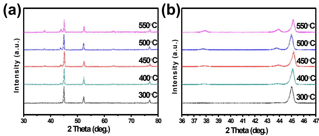
**Figure S3.** (a) The X-ray diffraction (XRD) pattern of the Ni(OH)<sub>2</sub> at different calcining temperatures from 300 to 500 °C for 1h. (b) Intensity variation diagram of characteristic peaks(43.3°) of NiO/NF.
