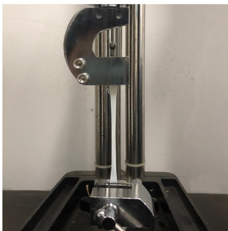
Figure S10. Photograph of the g-C 3 N 4 CSPE at stretch state.
