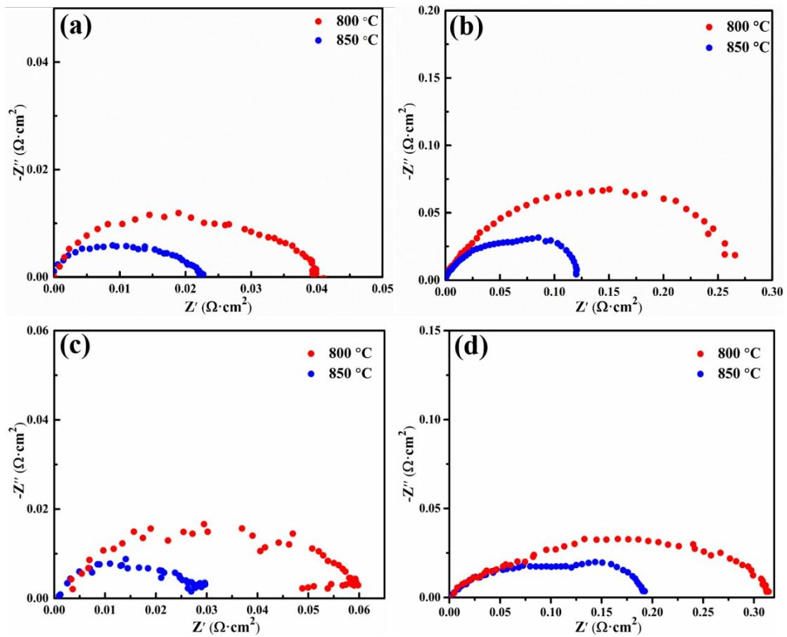
Figure. S2 EIS of LCaFN symmetrical cell tested in half cell mode at different temperature in air (a) and  $\text{CO}_2$  (b), LSrFN symmetrical cell at different temperature in air (c) and  $\text{CO}_2$  (d).
