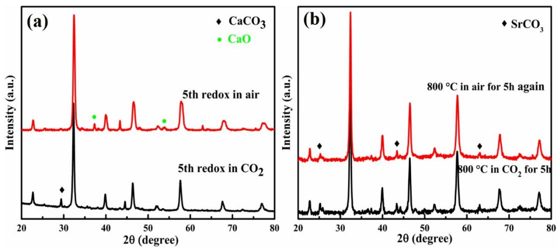
Figure. S1 X-ray diffraction patterns of LCaFN after five redox cycles at 800 °C in air and  $\text{CO}_2$  for 5 h (a), LSrFN treated in  $\text{CO}_2$  for 5 h and then treated in air for 5 h again (b).
