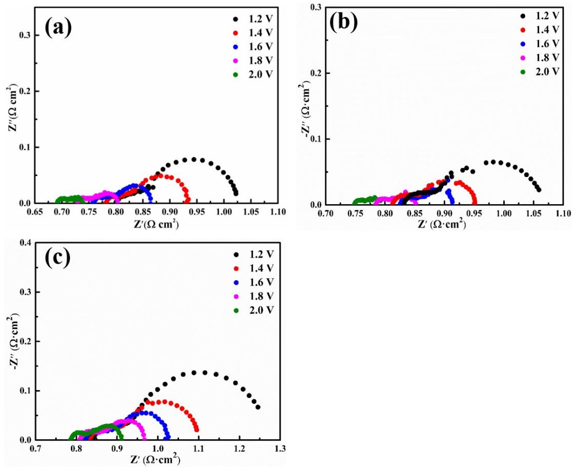
Figure. S5 Nyquist plots of LCaFN symmetrical cell (a), LCaFN asymmetrical cell (b) and LSrFN symmetrical cell (c) under different voltage (1.2~2.0 V) for pure  $\text{CO}_2$  electrolysis at 800  $^\circ\text{C}$ .
