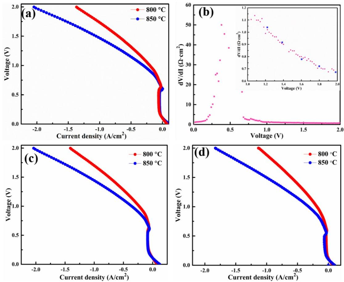
Figure. S3 I-V curves of the LCaFN symmetrical cell for pure CO<sub>2</sub> electrolysis at 800 °C and 850 °C (a) and the corresponding dV/dI-V curve at 800 °C (b). I-V curves of the LCaFN asymmetrical cell (c) and LSrFN symmetrical cell (d) for pure CO<sub>2</sub> electrolysis at 800 °C and 850 °C.
