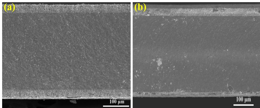
Figure. S7 SEM images of the LCaFN symmetrical cell before (a) and after (b) the electrolysis at 800 °C.
