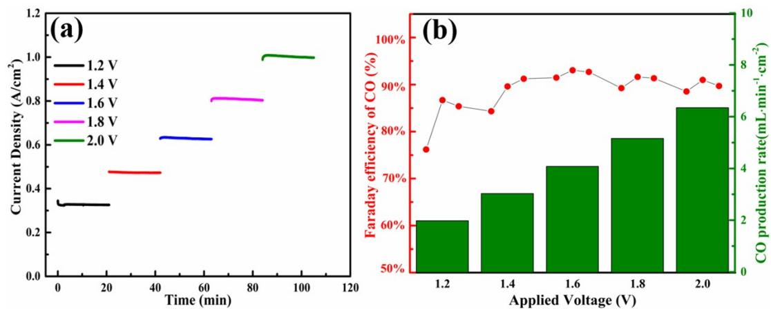
Figure. S6 Short-term performance of  $\text{CO}_2$  electrolysis at various voltage with LSrFN symmetrical cell (a); CO production rate and Faraday efficiency of LSrFN symmetrical cell (b) at 800 °C.
