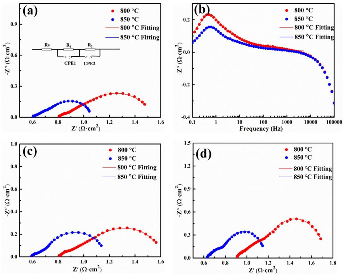
Figure. S4 Nyquist plot (a) and Bode plot (b) of the LCaFN symmetrical cell, Nyquist plots of LCaFN asymmetrical cell (c) and LSrFN symmetrical cell (d) for pure CO<sub>2</sub> electrolysis at 800 °C and 850 °C with fitting by equivalent circuit.
