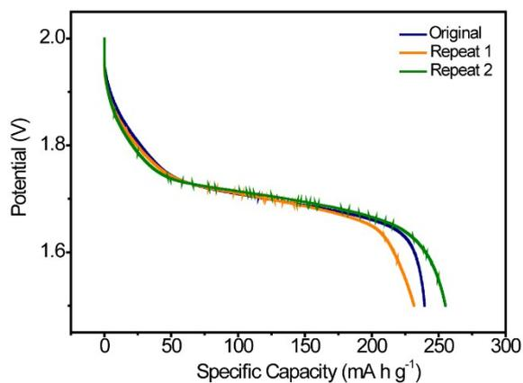
**Figure S7.** GCD curves at  $5.1 \text{ A g}^{-1}$  of  $\text{Ni}_3\text{S}_2@\text{PANI}//\text{Zn}$  battery in repeated experiments.
