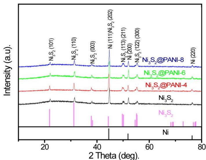
**Figure S1.** XRD patterns of pristine Ni<sub>3</sub>S<sub>2</sub>, Ni<sub>3</sub>S<sub>2</sub>@PANI-4, Ni<sub>3</sub>S<sub>2</sub>@PANI-6 and Ni<sub>3</sub>S<sub>2</sub>@PANI-8 electrodes.
