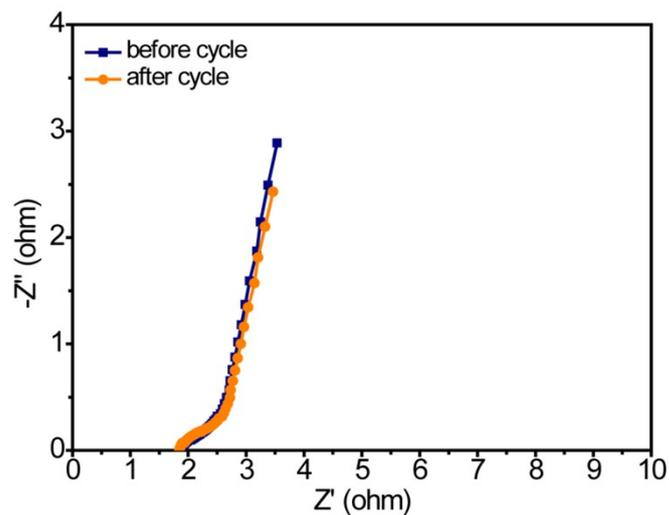
**Figure S8.** EIS spectra of  $\text{Ni}_3\text{S}_2@\text{PANI}//\text{Zn}$  battery before and after 5000 cycles.
