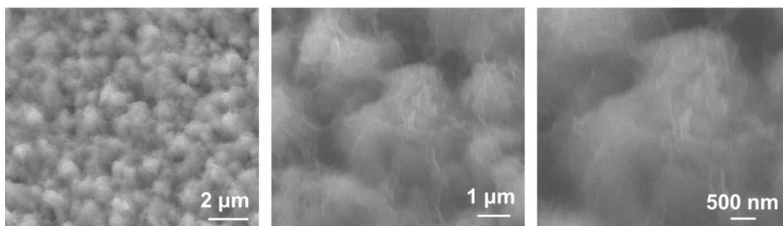
**Figure S4.** SEM images of  $\text{Ni}_3\text{S}_2@\text{PANI-6}$  electrode after 10000 cycles.
