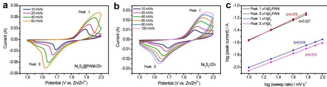
**Figure S9.** CV curves at various scan rates of (a)  $\text{Ni}_3\text{S}_2@\text{PANI}/\text{Zn}$ , (b)  $\text{Ni}_3\text{S}_2/\text{Zn}$ , and log (i) versus log (v) plots at specific peak currents.
