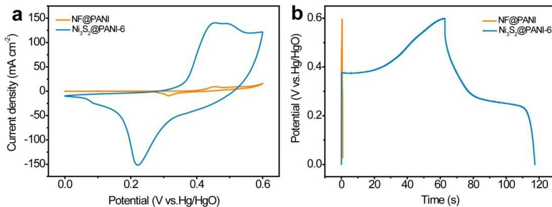
**Figure S5.** (a) CV curves at a scan rate of 10 mV s<sup>-1</sup>, (b) GCD curves at 14.2 A g<sup>-1</sup> of NF@PANI and Ni<sub>3</sub>S<sub>2</sub>@PANI-6 electrodes.
