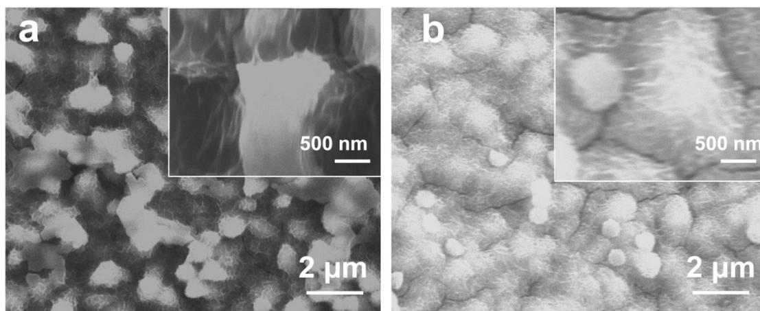
**Figure S2.** SEM images of the (a)  $\text{Ni}_3\text{S}_2@\text{PANI-4}$  and (b)  $\text{Ni}_3\text{S}_2@\text{PANI-8}$  electrodes (lower insets).
