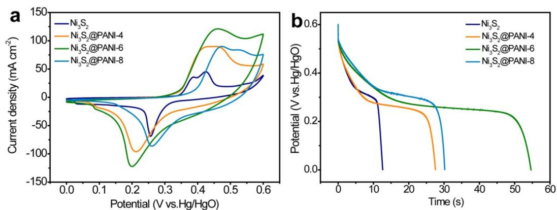
**Figure S3.** (a) CV curves at scanning rate of  $10 \text{ mV s}^{-1}$ , (b) GCD curves at  $14.2 \text{ A g}^{-1}$  of the  $\text{Ni}_3\text{S}_2$ ,  $\text{Ni}_3\text{S}_2@\text{PANI-4}$ ,  $\text{Ni}_3\text{S}_2@\text{PANI-6}$  and  $\text{Ni}_3\text{S}_2@\text{PANI-8}$  electrodes.
