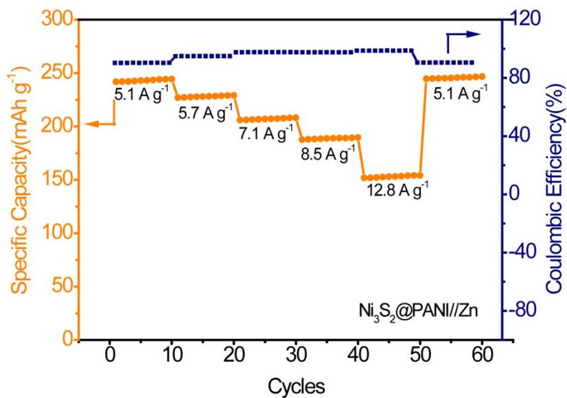
**Figure S6.** The rate performance of Ni<sub>3</sub>S<sub>2</sub>@PANI//Zn battery.
