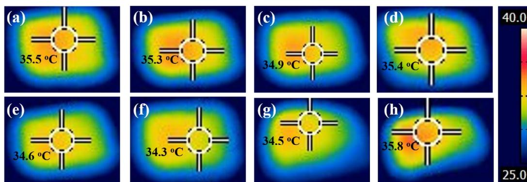
**Figure S5.** IR image of the PB3@CF surface for different solvents evaporation under one sun illumination, (a) acetone, (b) toluene, (c) ethanol, (d) water, (e) n-propanol, (f) DMAC, (g) n-hexanol, (8) NMP
