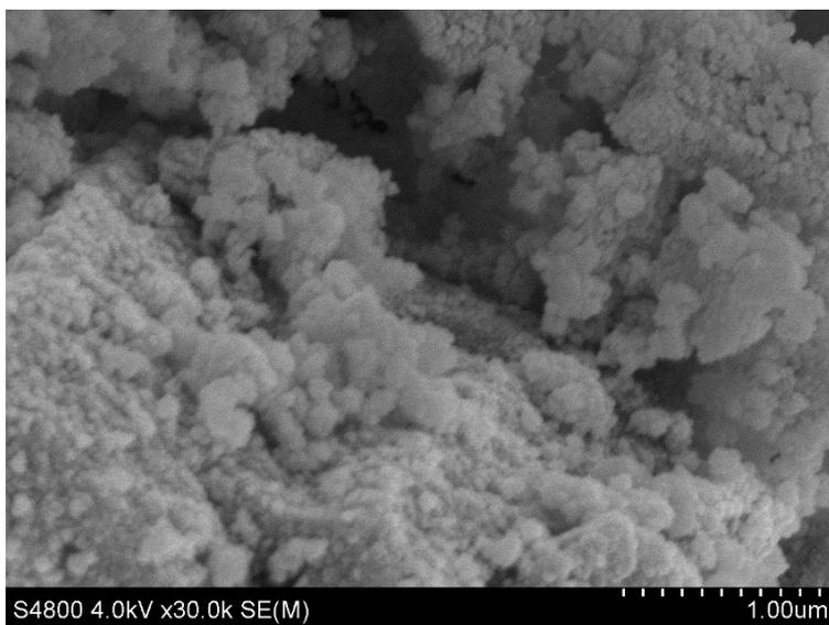
**Figure S2.** SEM image of PB powder prepared from conventional coprecipitation of  $\text{Fe}^{3+}$  and  $\text{Fe}(\text{CN})_6^{4-}$ .
