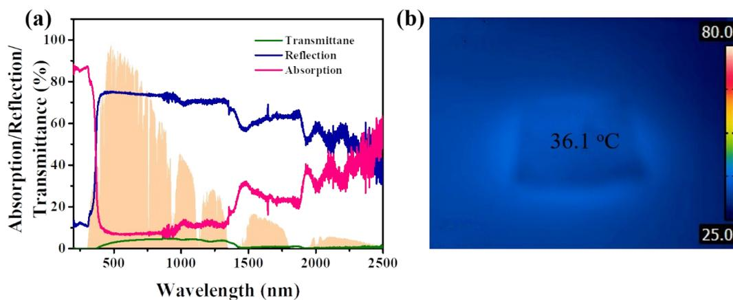
**Figure S4.** (a) Transmittance, reflection and absorption curves of bare CF; (b) IR image of the bare CF surface under one sun illumination.
