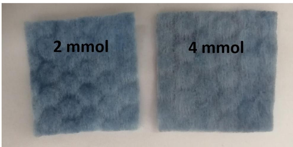
**Figure S3.** Photograph of the obtained PB@CF prepared from different precursor concentration of  $\text{Na}_4\text{Fe}(\text{CN})_6$ .
