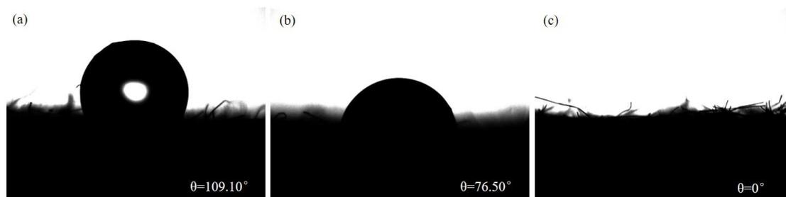
**Fig. S4** Contact angle measurement of the (a) pristine graphite felt, (b) thermally treated graphite felt and (c) gradient-pore graphite felt.
