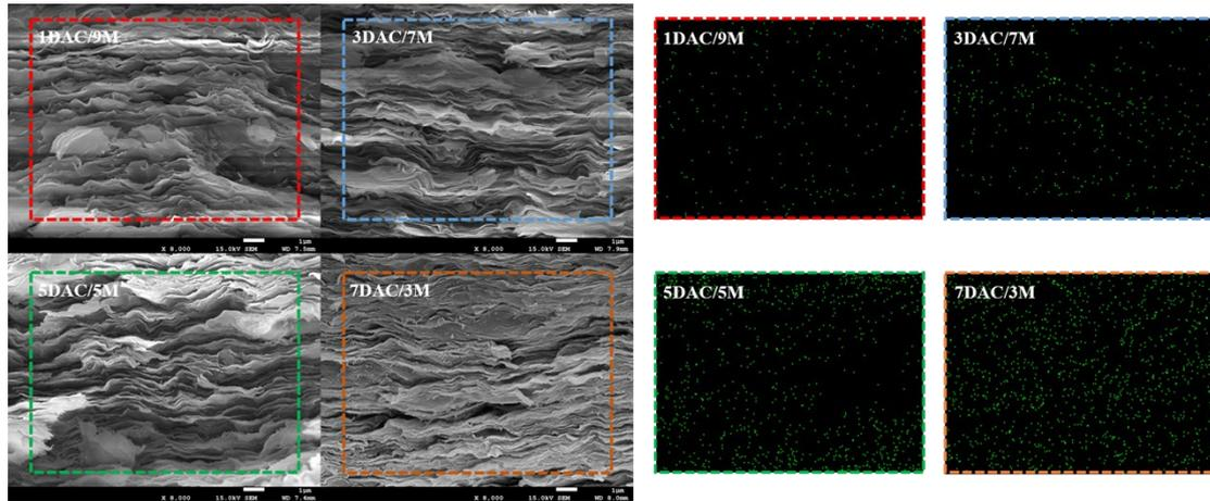
**Figure S3.** SEM-EDS mapping indicating uniform distribution of nitrogen in composite film.
