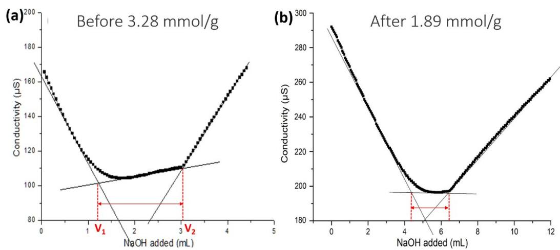
**Figure S1.** Conductometric titration curve for (a) CMC and (b) DA-CMC3
