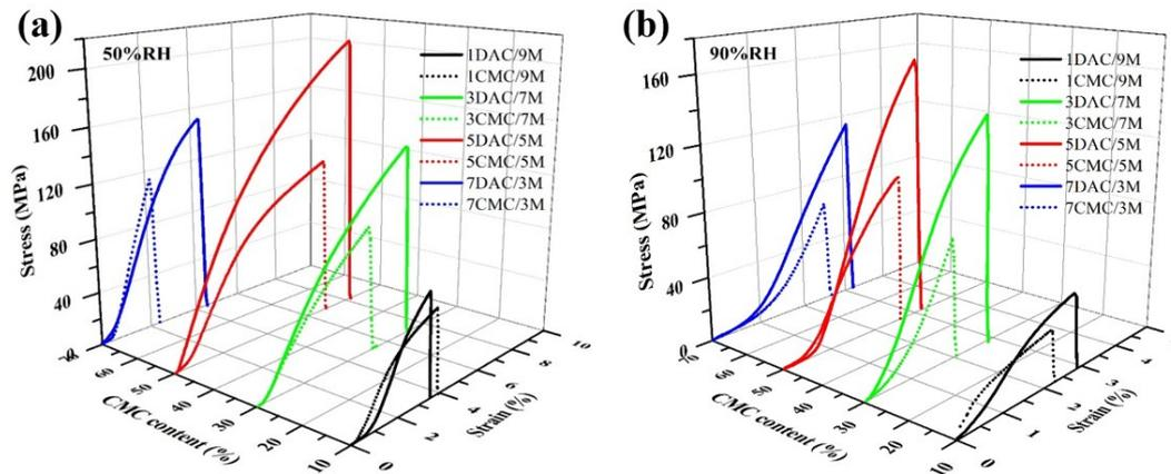
**Figure S5.** Representative stress-strain curves from tensile test at the relative humidity of (a) 50% and (b) 90%.
