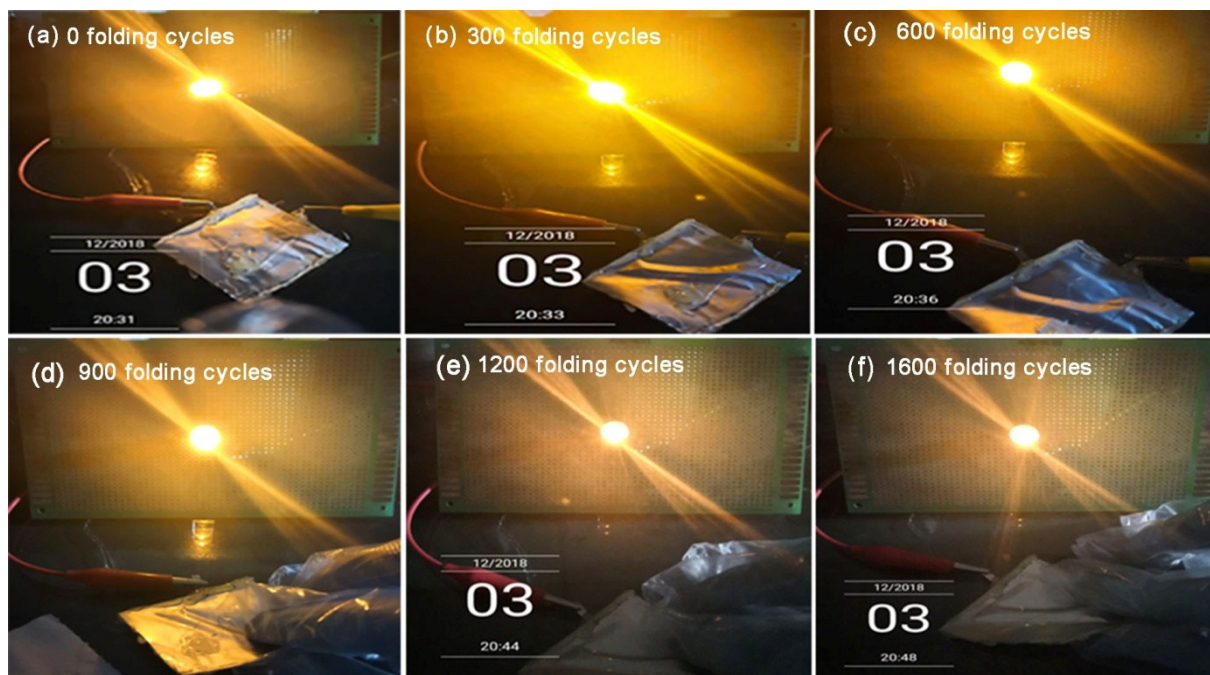
Fig. S2 Photographs of the pouch-type FSIFB assembled with the BFCF-NVP/HCF cathode and the PGN/SiC/HCF anode, showing different luminosity of lighted LED bulb driven by the FSIFB after different bending cycles in a bending angle of 30–90°.
