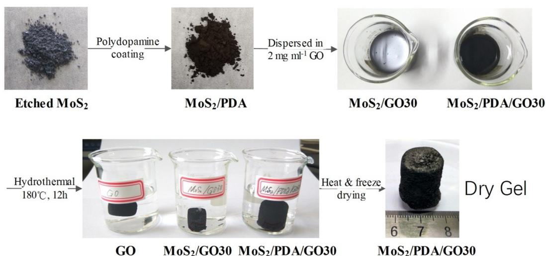
Figure S1. Schematic diagram of the detailed synthesis route of MoS<sub>2</sub>-PDA-GO30.
