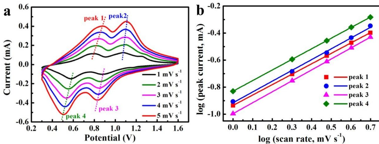
Figure S10 The CV curves of  $V_2O_5//Zn$  battery at various scan rates.
