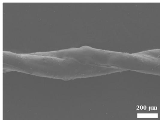
**Figure S7** The SEM image of the assembled fiber-shaped Zn-ion battery.
