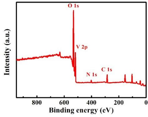
**Figure S4** The XPS spectrums (Fig. SX) of CNTF@NC@V<sub>2</sub>O<sub>5</sub>.
