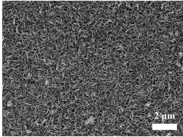
**Figure S3** The SEM images of CNTF@V<sub>2</sub>O<sub>5</sub>.
