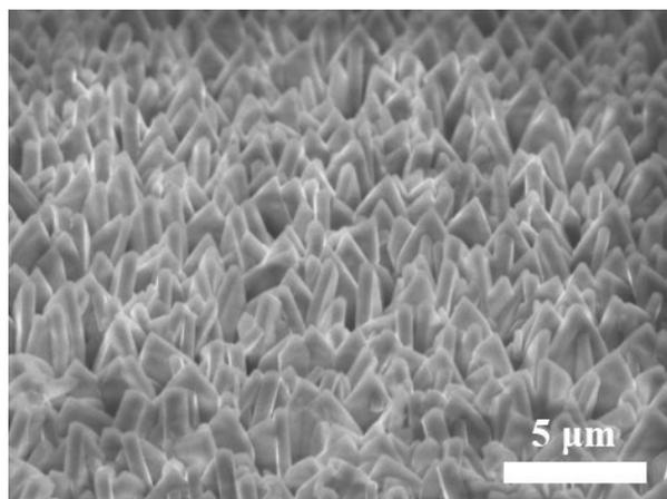
**Figure S1** The SEM image of CNTF@Co-MOF.
