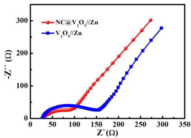
**Figure S12** The Nyquist plots of NC@V<sub>2</sub>O<sub>5</sub>//Zn and V<sub>2</sub>O<sub>5</sub>//Zn batteries.
