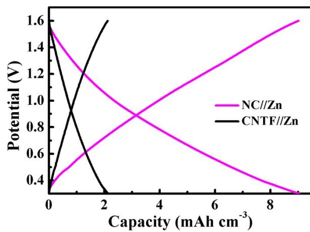
**Figure S8** The GCD curves of CNTF//Zn and CNTF@NC//Zn batteries at a current density of 0.3 A cm<sup>-3</sup>.
