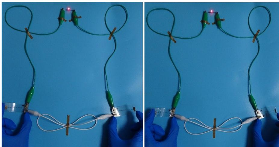
**Figure S14** A LED powered by two fiber-shaped batteries in series under various bend angles.
