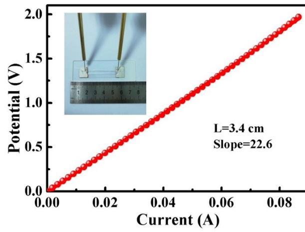
**Figure S11** Current-voltage characteristic curve of the CNTF@NC@V<sub>2</sub>O<sub>5</sub>.
