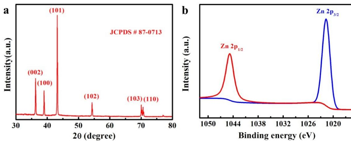
**Figure S6** The XRD pattern and XPS spectrum of Zn nanosheets.
