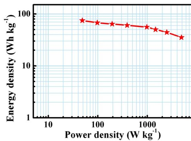
**Figure S13** Specific energy and power densities of the device.
