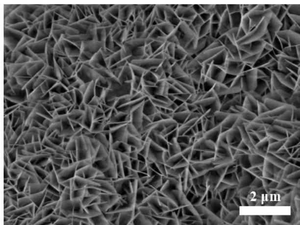
**Figure S5** The SEM image of CNTF@Zn.
