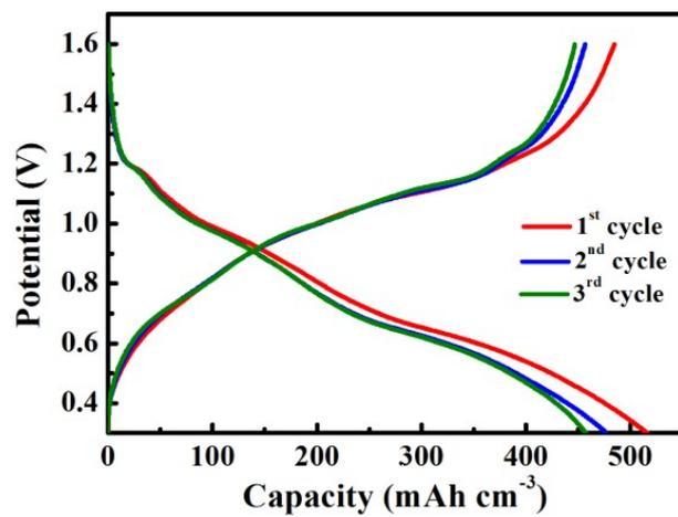
**Figure S9** The GCD curves of initial three cycles for the NC@V<sub>2</sub>O<sub>5</sub>//Zn battery.
