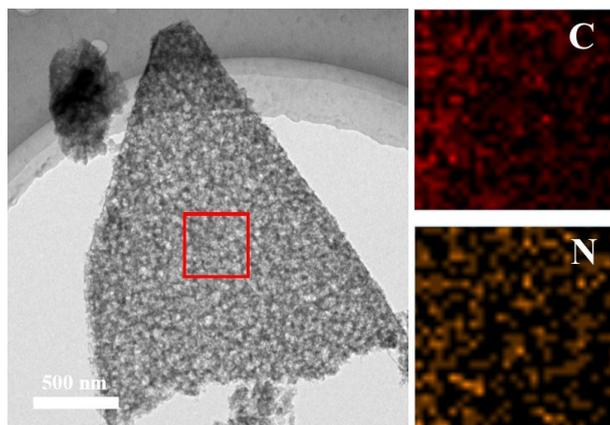
**Figure S2** EDX mappings of C and N elements measured from NC nanowall.
