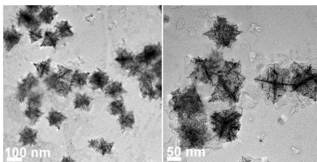
**Figure S2.** Low-magnification TEM image of PtCu-O EOND nanostructures.
