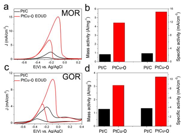
**Figure S13.** Specific activity and mass activity of commercial Pt/C and PtCu-O EOUDs for methanol (a, b) and glycerol (c, d) at a scan rate of  $50 \text{ mV s}^{-1}$ .
