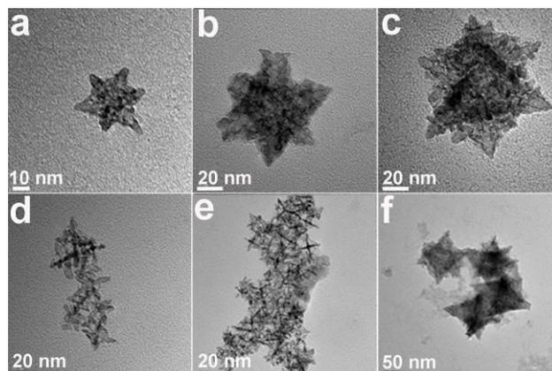
**Figure S6.** TEM images of the PtCu-O nanostructures formed after different reaction times. a, d) 2 h, b, e) 2.5 h, and c, f) 3 h.
