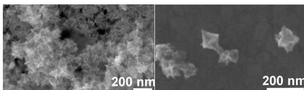
**Figure S15.** SEM images of PtCu-O nanostructures after catalytic operation.
