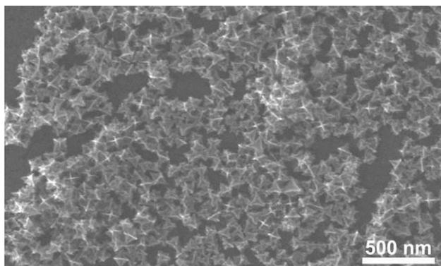
**Figure S1.** Low-magnification SEM image of PtCu-O EOND nanostructures.
