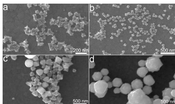
**Figure S8.** SEM image of PtCu-O nanostructures obtained with different amount of ethanolamine in the synthesis while keeping the other parameters constant. a) 0.3 ml b) 0.5 ml c) 0.7 ml d) 0.9 ml.
