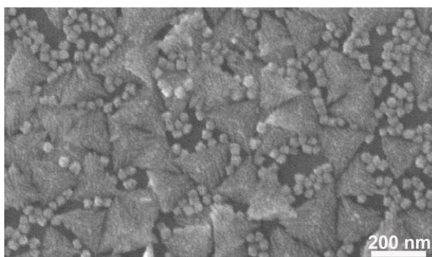
**Figure S7.** SEM image of PtCu-O nanostructures obtained without the addition of ethanolamine in the synthesis while keeping the other parameters constant.
