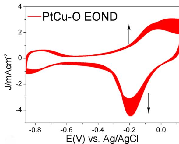
**Figure S12.** Activated CV curves of PtCu-O EOUD nanostructures in 0.5 M KOH solution for 100 cycles.
