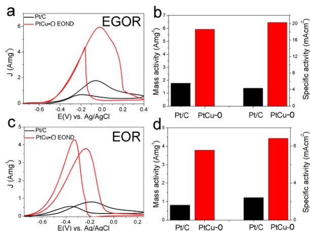
**Figure S14.** Specific activity and mass activity of commercial Pt/C and PtCu-O EOUDs for ethylene glycol (EGOR) (a, b) and ethanol (EOR) (c, d) at a scan rate of  $50 \text{ mV s}^{-1}$ .
