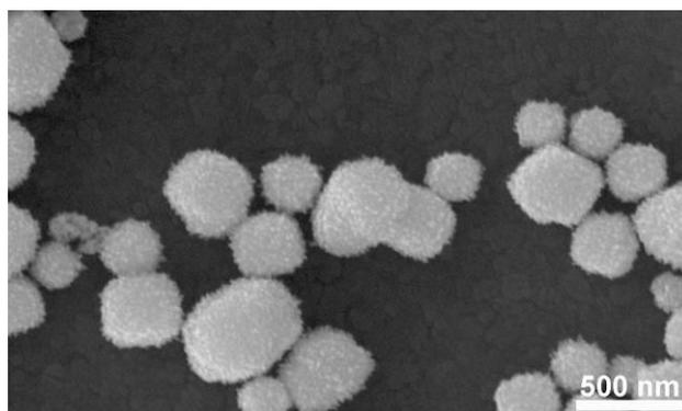
**Figure S10.** SEM image of Pt nanoparticles obtained without the addition of  $\text{CuCl}_2$  in the synthesis while keeping the other parameters constant.
