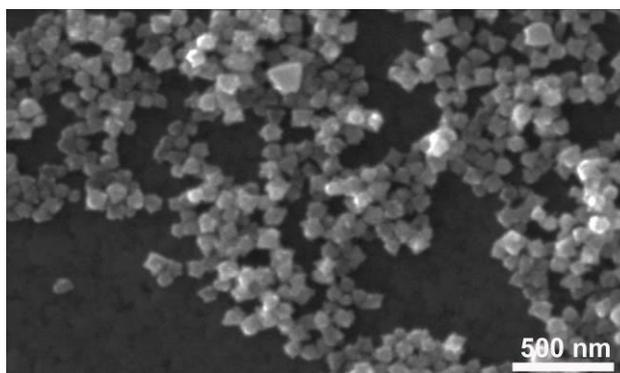
**Figure S9.** SEM image of PtCu-O nanostructures obtained without the addition of acetamide in the synthesis while keeping the other parameters constant.
