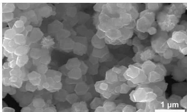
**Figure S11.** SEM image of PtCu-O nanostructures obtained without the addition of KI in the synthesis while keeping the other parameters constant.
