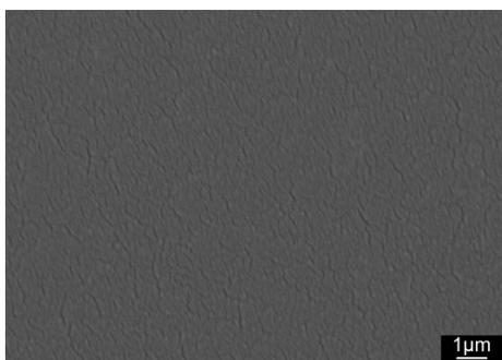
Figure S12. SEM image of the tensile fracture surface of XSBR
